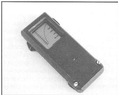
The Edge, manufactured by Orca Industries, was one of the first microprocessor-based dive computers used extensively by recreational divers.
