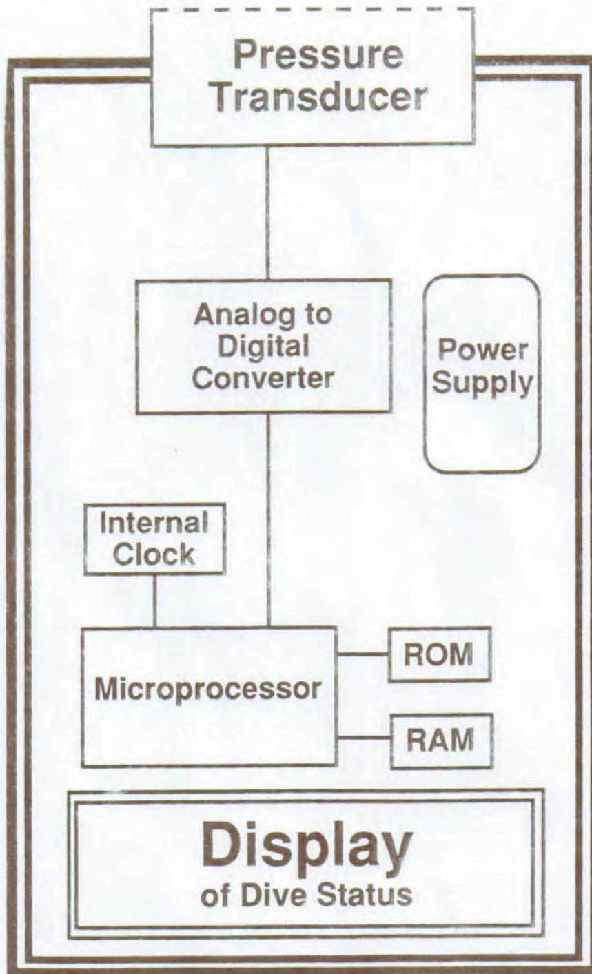
Figure 1. Dive Computer Schematic
