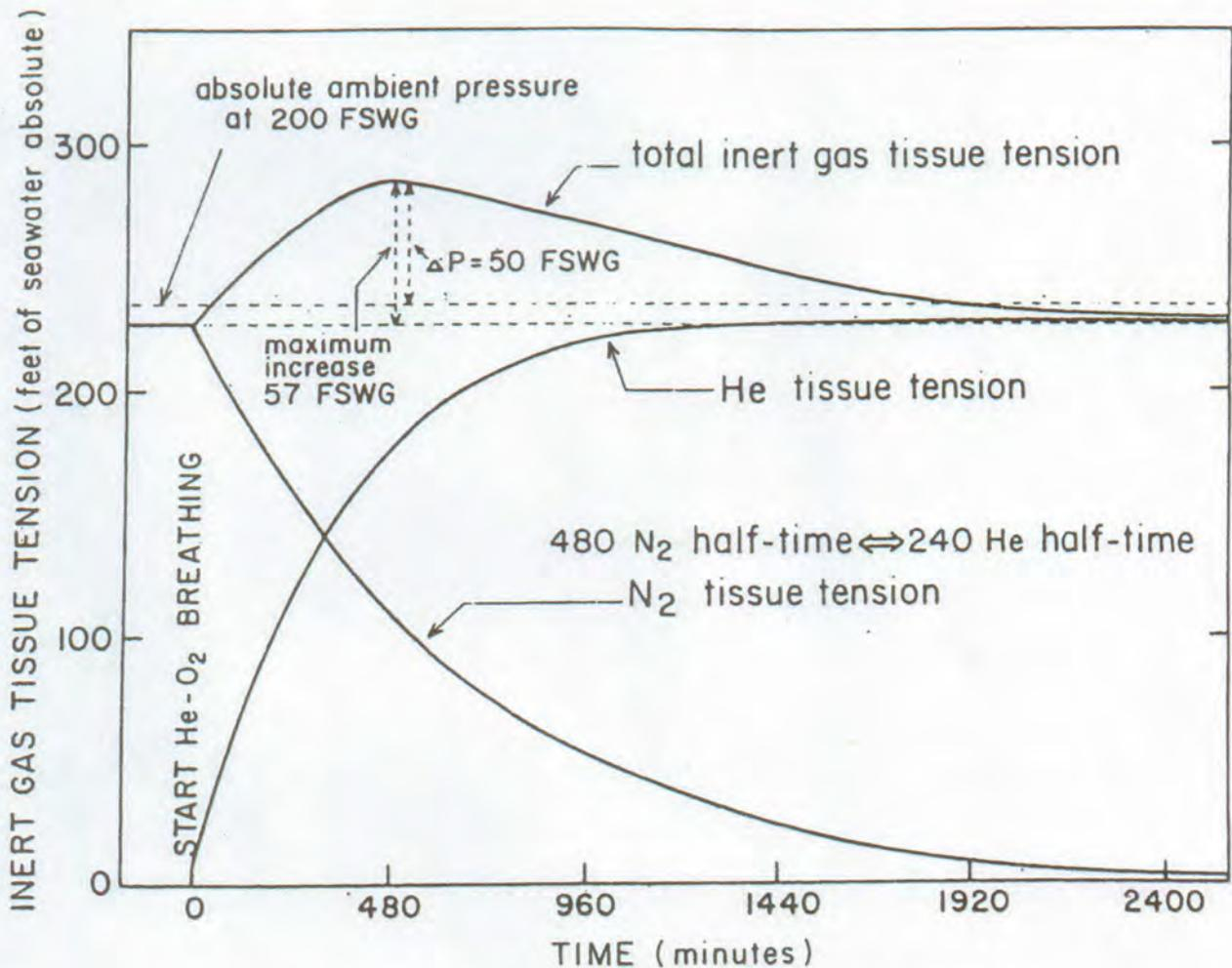
Figure 2. Isobaric Counterdiffusion and Supersaturation
