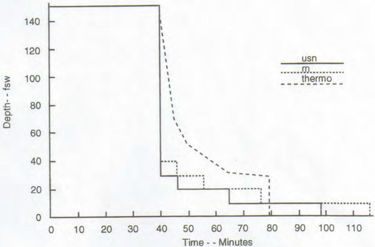
Figure 3. Thermodynamic Staging Versus USN and RN Staging
