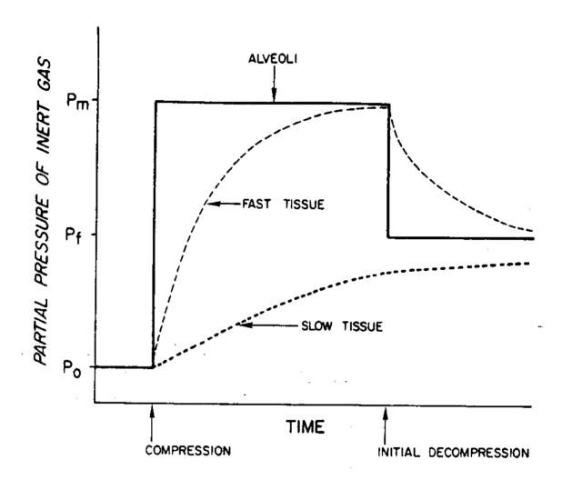
Fig. 1 - Response of fast and slow tissues exposed to a rectangular pressure schedule consisting of a rapid compression from an initial pressure P to some maximum pressure P and a rapid decompression to an intermediate pressure  $P_{\bf f}$ .
