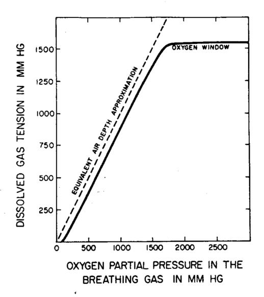
Fig. 4 - Plot of dissolved gas tension versus oxygen partial pressure. The equivalent-air-depth approximation is useful for oxygen partial pressures below 1500 mm Hg.
