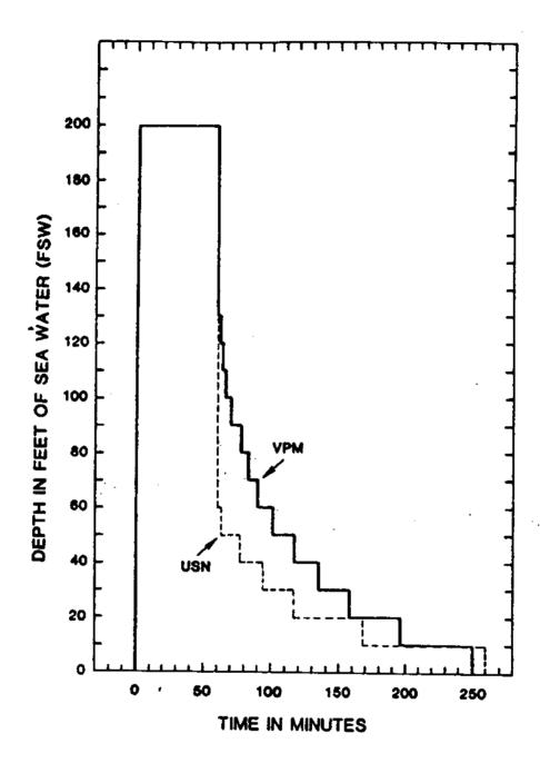
Fig. 8 - Plot of VPM and USN decompression profiles for a 60-Min, 200-fsw air excursion. The longer "first pull" of conventional air tables results in a larger supersaturation, a larger bubble number, and a larger maximum volume of released gas.
