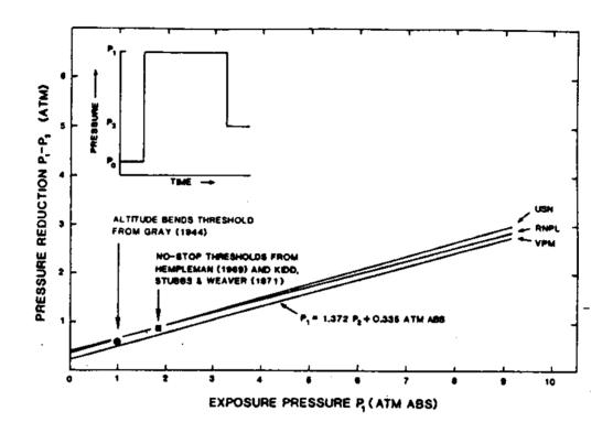
Fig. 12 - Plot of allowed pressure reduction versus exposure pressure for VPM, USN, and RNPL air tables. The VPM line lies below the no-stop and altitude bends thresholds and is therefore assumed to be "safer."
