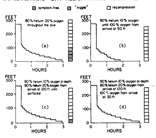
Fig. 22 - Four 20-min, 270-fsw excursions on various gas mixtures. Note the benefit of the oxygen stages in schedules (b) and (d). (Adapted from Elliott [62]).
