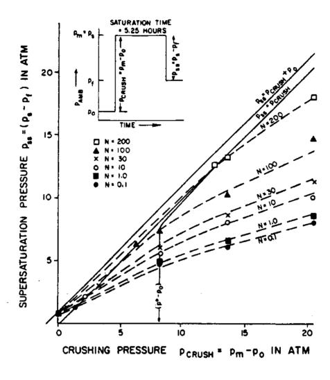
Fig. 2 - Plot of supersaturation versus crushing pressure for various lines of constant bubble number. The sudden decrease in slope at  $P_{\rm crush}$  = 8.2 atm indicates the onset of impermeability.
