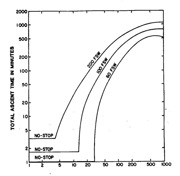
Fig. 21 - Plot of VPM residual-nitrogen helium total ascent times versus bottom times for 60, 100, and 200-fsw dives. The more-restrictive limits shift the curves to the left of those in Fig. 18.
