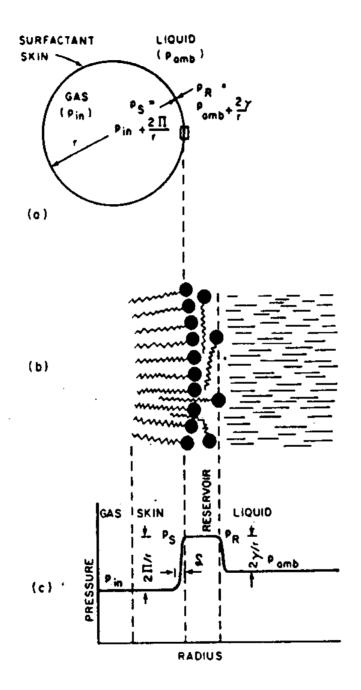
Fig. 15 - Schematic diagram of a bubble nucleus including: (a) the condition for mechanical equilibrium against small fluctuations, (b) a magnified view of the skin and the reservoir, and (c) a plot of pressure versus radius indicating where  $P_{in}$ ,  $P_{S}$ ,  $P_{R}$ , and  $P_{amb}$  apply.
