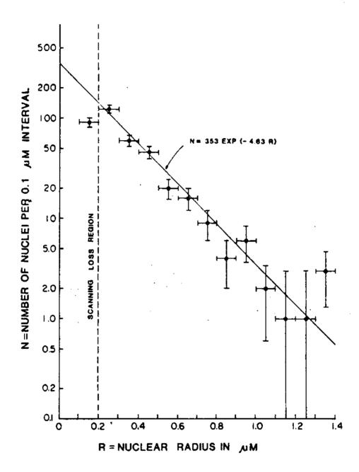
Fig. 3 - Differential radial distribution of gas cavitation nuclei in agarose gelatin. Above 0.2  $\mu$ m, the points can be described by a decaying exponential. Below 0.2  $\mu$ m, the microscope scanning efficiency deteriorates rapidly, and data in this region should be disregarded.
