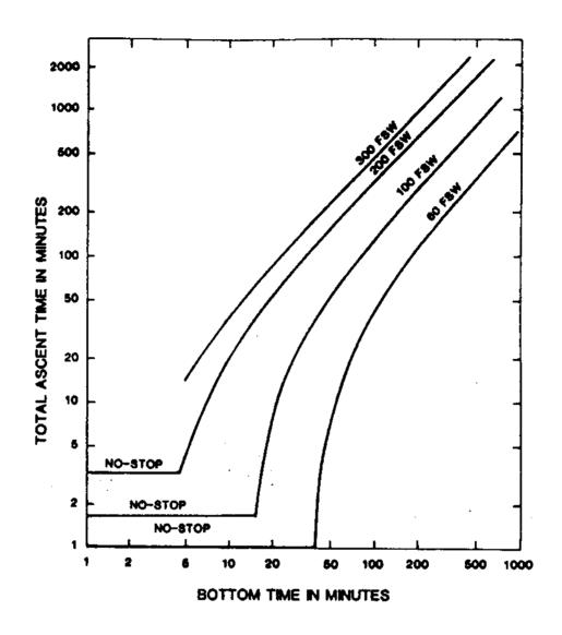
Fig. 11 - Plot of VPM total ascent times versus bottom times for 60, 100, 200, and 300-fsw air excursions. This figure illustrates how a two-dimensional map of decompression experience can be described by a global theory using a small number of equations and parameter values.
