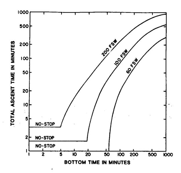
Fig. 18 - Plot of VPM total ascent times versus bottom times for 60, 100, and 200-fsw helium SCUBA excursions. The global map allows an instant comparison to be made with new helium data.
