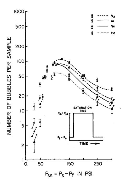
Fig. 13 - Plot of bubble number versus supersaturation pressure for various inert gases. The bubble number curves for helium and nitrogen are quite similar over the entire range of supersaturation pressures.
