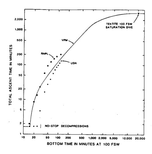
Fig. 10 - Plot of total ascent times versus bottom times for VPM, USN, and RNPL at 100 fsw on air. The VPM line lies comfortably between the USN and RNPL points for similar exposures, yet it spans the entire range from no-stops to saturation dives with the same four parameters.
