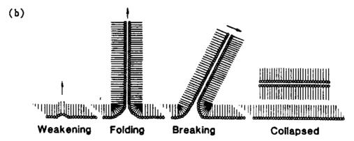
Fig. 14 - Behavior of compressed monolayers: (a)  $\Pi$ -A curves for typical synthetic phospholipids on a phosphate buffer (pH 7.4) at 21-24 °C. Curves 1, 3, and 5 are lecithins, while curves 2 and 4 are phosphatidylethanolamines. (b) A proposed mechanism for monolayer collapse. In the varying-permeability model,  $\Pi$  is replaced by the constant  $\gamma_C$ .
