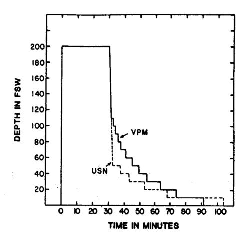
Fig. 17 - Plot of VPM and USN decompression profiles for a 30-Min, 200-fsw helium exposure. The VPM first stops are typically much deeper than their USN counterparts.
