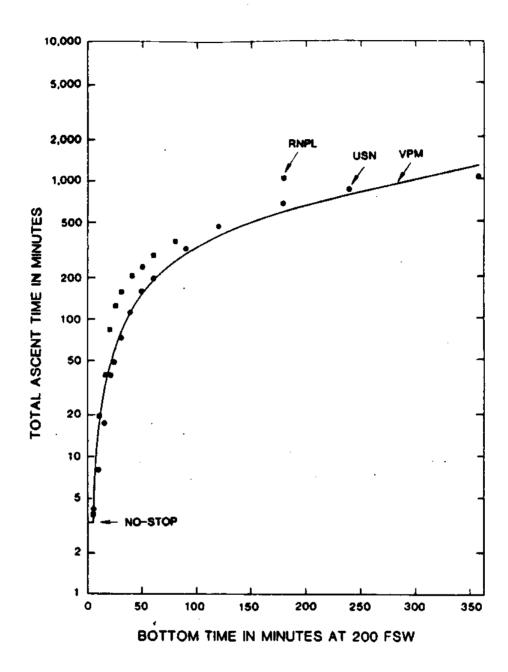
Fig. 9 - Plot of total ascent times versus bottom times at  $200~\rm{fsw}$  for the VPM, RNPL, and USN air tables. The total ascent times for the USN and RNPL air tables often differ by more than a factor of two.
