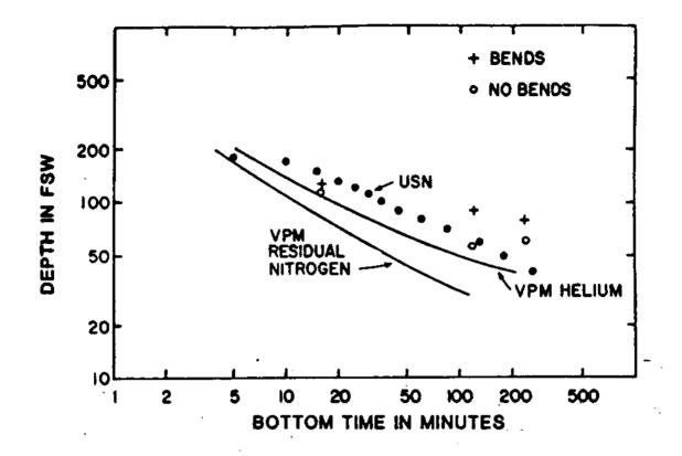
Fig. 19 - Plot of VPM residual nitrogen, VPM helium, and USN no-stop decompression limits. Several data points are included for reference. The VPM residual nitrogen curve lies in the safer region below the USN points and regions of bends incidence.
