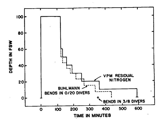
Fig. 20 - Plot of VPM residual nitrogen and Buhlmann's schedules for a 120-min, 100-fsw excursion. The profiles are quite similar, but the VPM total time is farther from the bends threshold.
