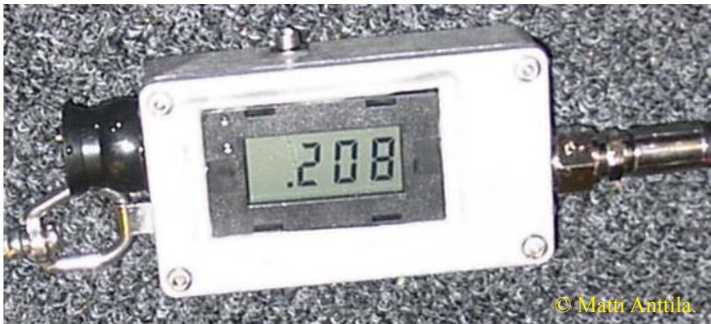
The ppO2 handset I added to the original device. Don't use the IDA-59 without this.
