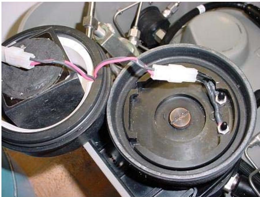
Figure 21. Improperly spliced connectors in an electronics pod.
