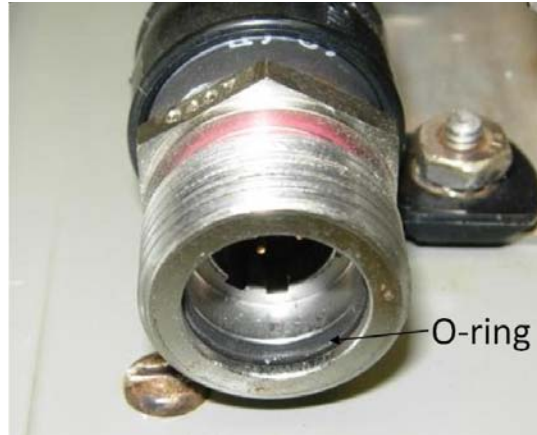
Figure 20. A damaged O-ring in this connector contributed to a fatality.
