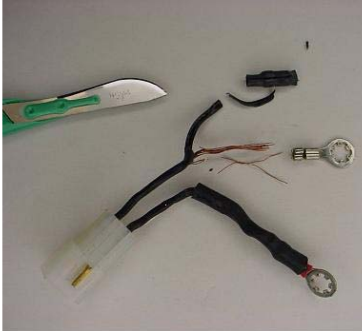
Figure 22. Connecting wires damaged by improper repair.
