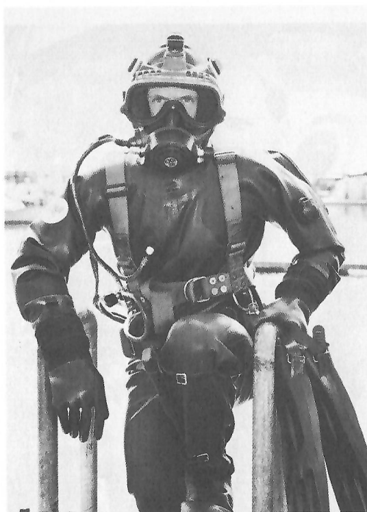
Fig. 1.1 Full face masks like the EXO-26® are designed to cover the entire face, but not the head.
