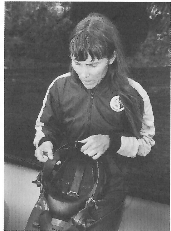
Fig. 5.9 Always check the spider carefully prior to dressing in.
