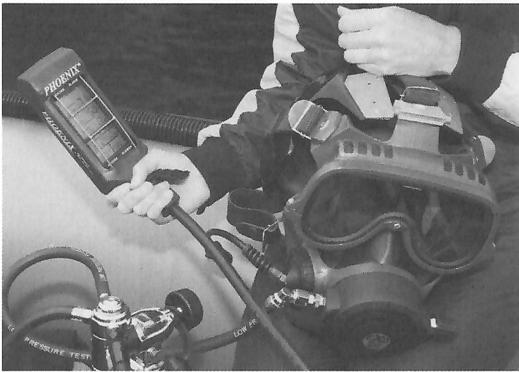
Fig. 5.3 An electronic pressure gauge and dive computer like ORCA's Phoenix is very useful when diving with a full face mask. This unit will tell you how much bottom time you have left based upon your present air consumption.
