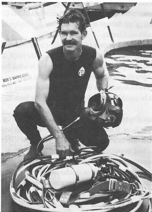
Fig. 1.5 The EXO-26® can be used for surface supplied diving as well as with scuba.
