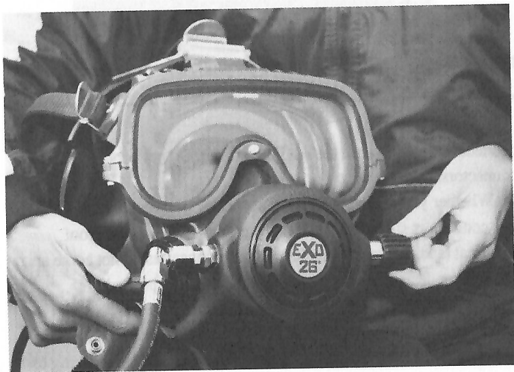
Fig. 5.10 Make sure the regulator adjustment knob is functioning properly prior to diving.
