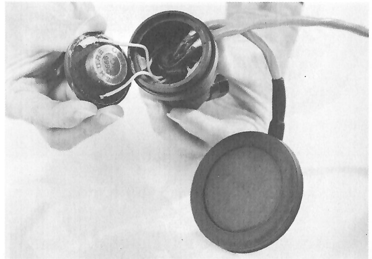
Fig. 8.1 Removing the microphone from the DSI communications module.
