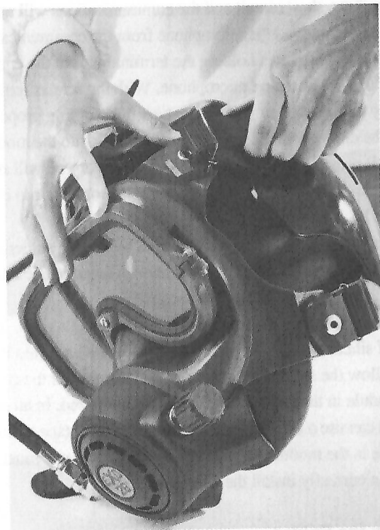
Fig. 8.3 Replacing the spider.
