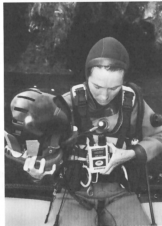
Fig. 1.3 The addition of wireless communications allows divers wearing full face masks to communicate with each other.
