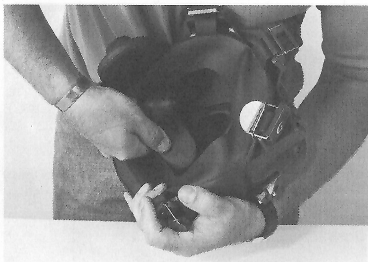
Fig. 7.6 Remove the air delivery tube prior to rinsing.
