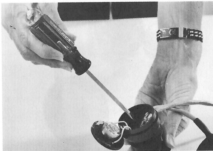
Fig. 8.2 Loosening the screws that hold the communications components in the module.
