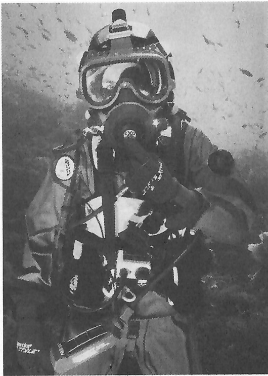
Fig. 5.18 To clear the mask of water, push the purge button on the front of the regulator.
