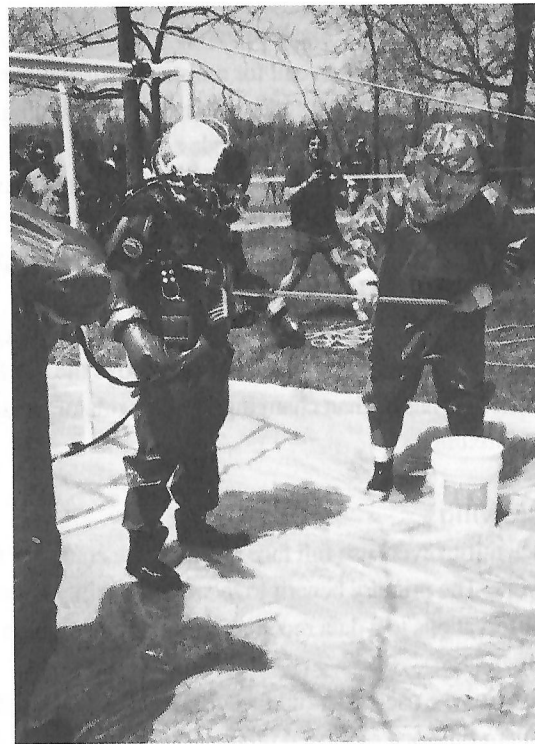
Fig. 1.6 In some contaminated water situations, a helmet like the SuperLite-17® may be the best choice for diving operations.
