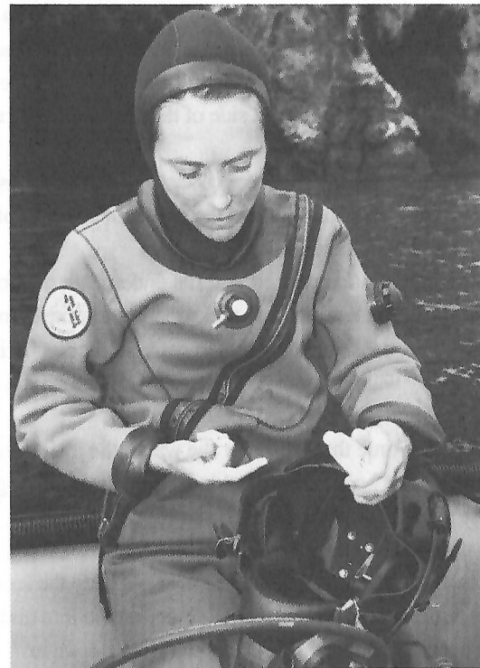
Fig. 5.11 You may want to apply a bit of soap to the lens to help keep the mask from fogging up.
