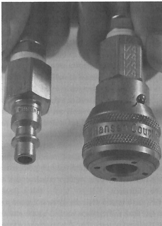
Fig. 3.2 Close-up view of quick disconnect fittings with a sleeve lock on the female fitting.
