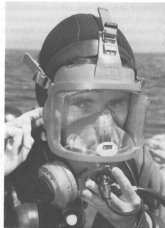
Fig. 5.22 Test the positive pressure system prior to entering the water.
