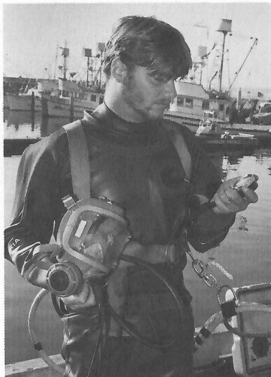
Fig. 6.13 Be sure to check the pressure in the bail-out bottle before you enter the water.
