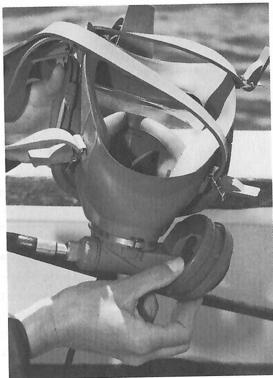
Fig. 5.19 Make sure the lever that controls the positive pressure is pushed in (closed) before you turn the air on to the mask, if you are using the positive pressure second stage.
