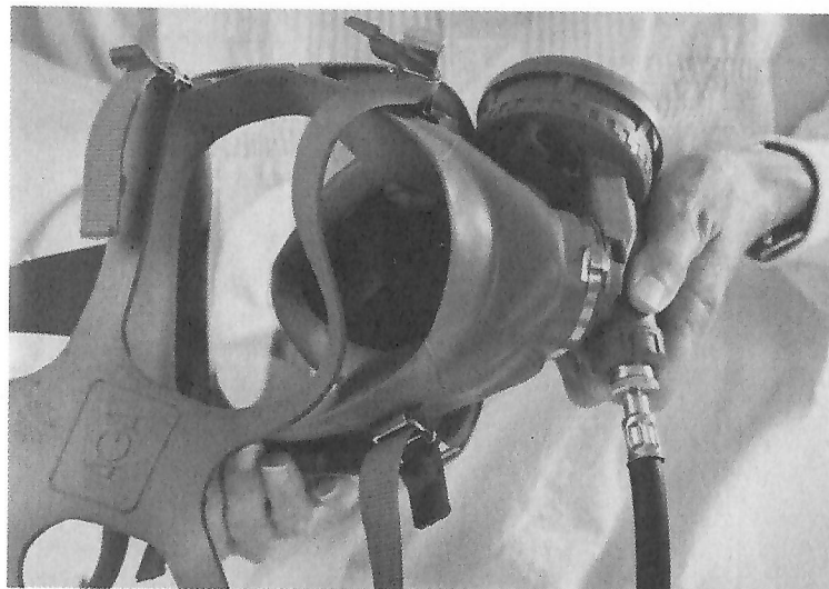
Fig. 7.2 After the microphone has been removed, hold the mask in one hand and twist the regulator with your other hand to remove it.
