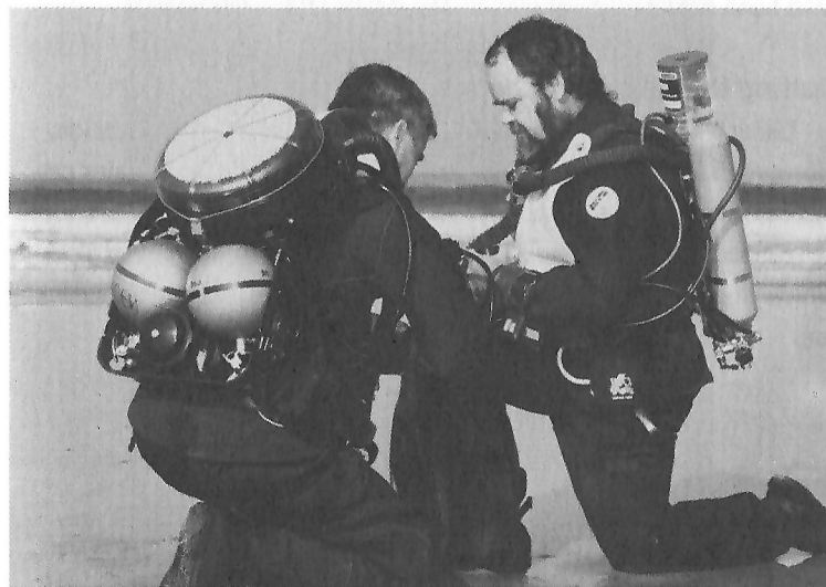
Fig. 1.8 A full face mask may be a better choice for deep technical diving, such as might be done with a closed circuit rig like the equipment shown here.
