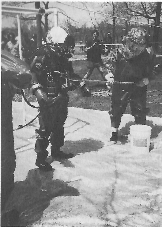
Fig. 1.7 In some contaminated water situations, a helmet like the SuperLite-17® may be the best choice for diving operations.
