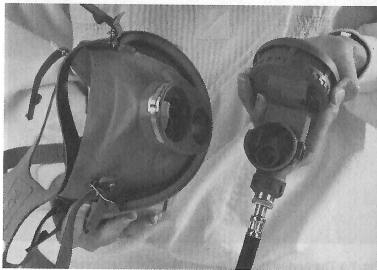
Fig. 7.3 The regulator is easily separated from the mask.
