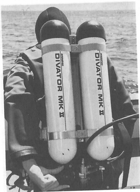
Fig. 5.9 Locate the valve handle to turn the air on by reaching back behind you with your left hand.
