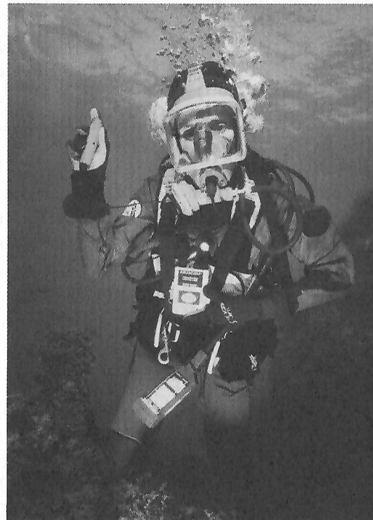
Fig. 2.1 Communications are one of the big advantages of using a full face mask like the Divator MK II.
