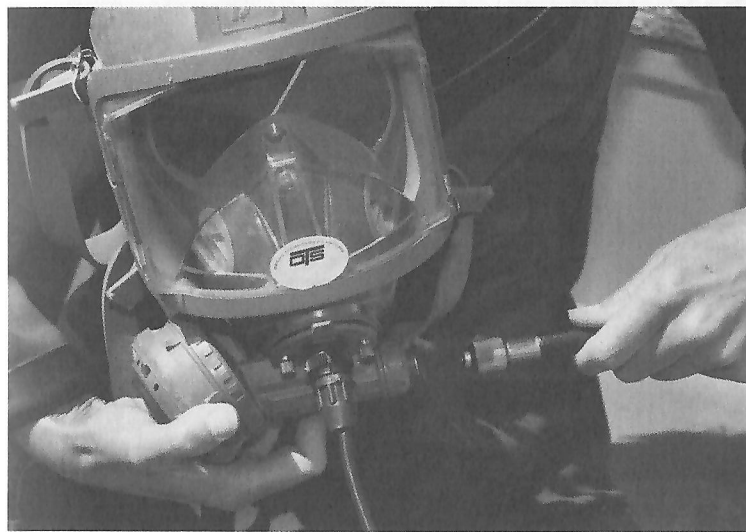
Fig. 5.3 Connect the low pressure hose to the mask.
