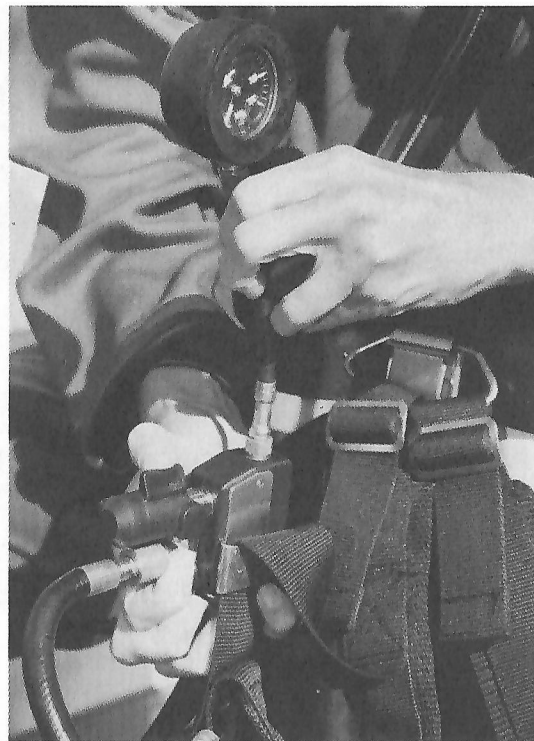
Fig. 5.8 You cannot access the reserve air until the cylinder pressure drops to 1125 P.S.I. or less, if you are using 4500 P.S.I. cylinders.
