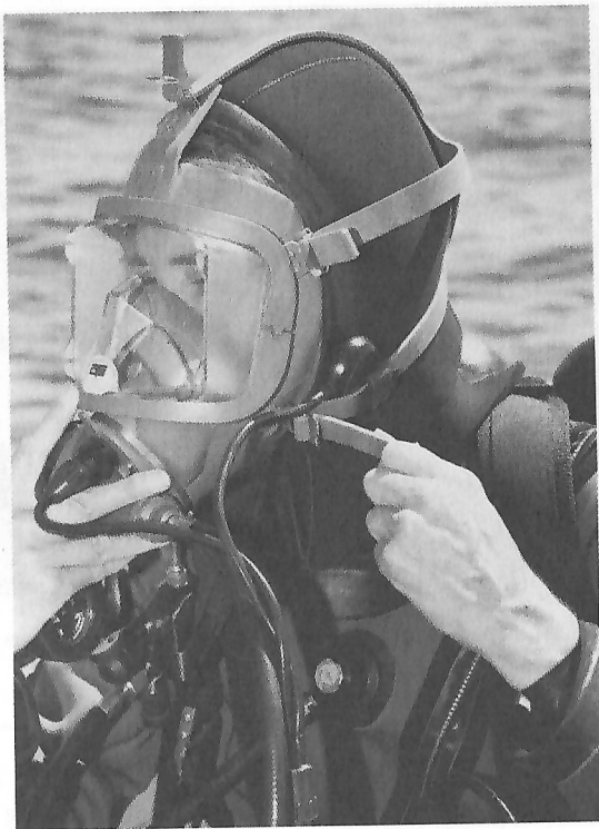
Fig. 5.11 Correct positioning for the earphone.
