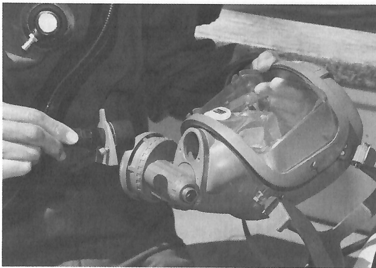
Fig. 7.1 Remove the microphone prior to rinsing the mask.
