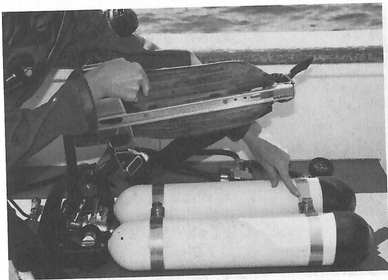
Fig. 5.4 Mount the backpack to the cylinders with the small end of the pack away from the valve.
