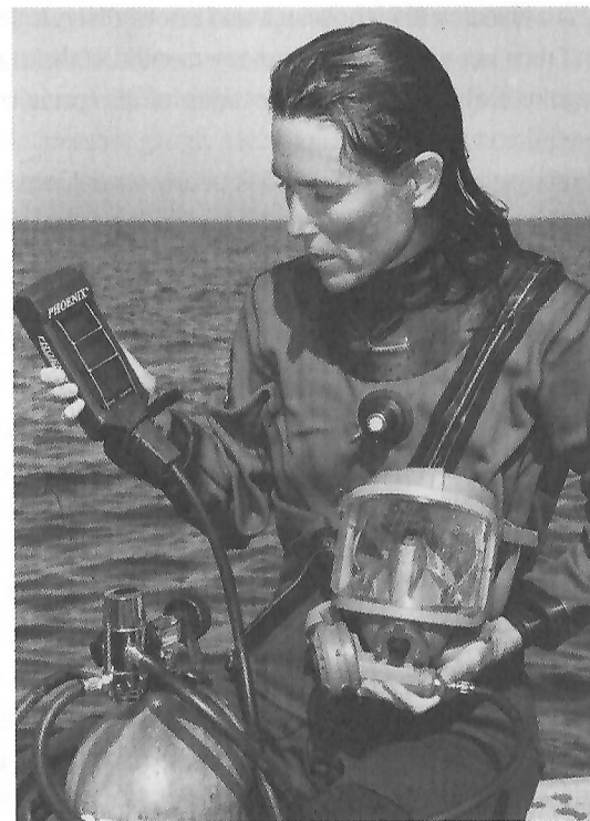
Fig. 5.1 An electronic pressure gauge and dive computer like ORCA's Phoenix is very useful when diving with a full face mask. This unit will tell you how much bottom time you have left based upon your present air consumption.
