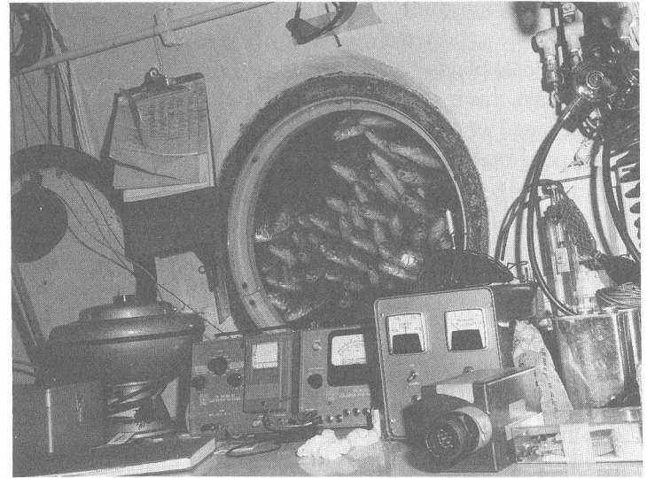
A night view out the Sealab port. The array of devices includes atmosphere monitoring equipment and a centrifuge for blood studies. (U.S. Navy photo)
