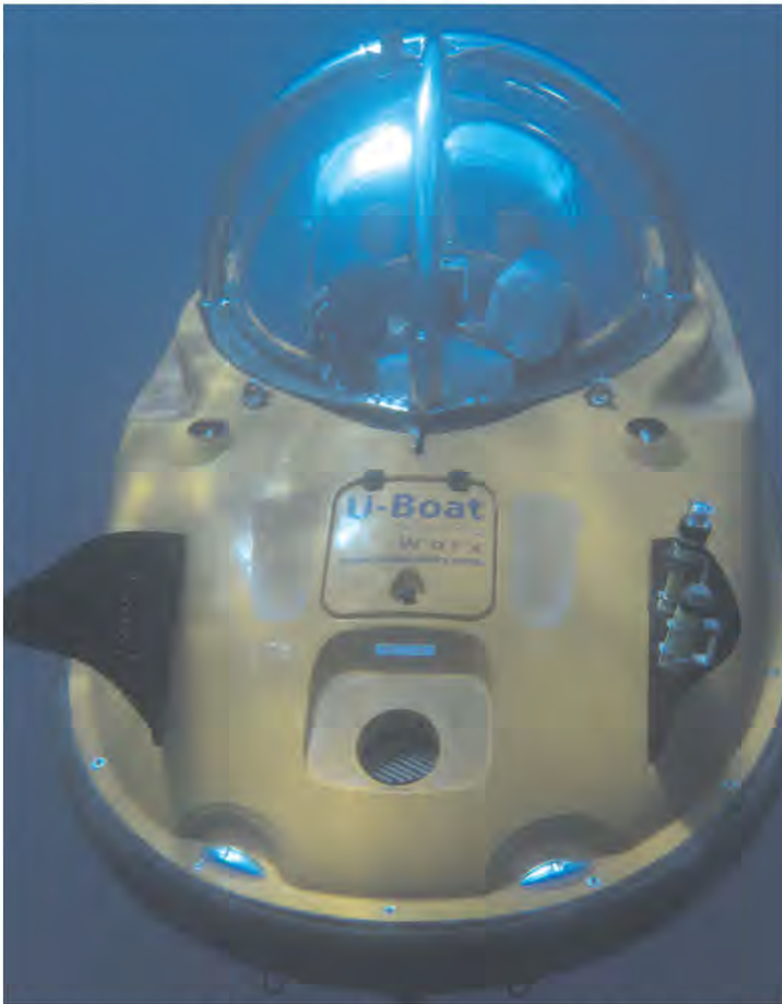
Figure 5.4. Uboatworx’s C-Quester is a dedicated super-yacht submersible based on a double-hull configuration known as the Underwater Boat Concept. The first hull is the exostructure that ensures excellent stability, while the second hull is the actual pressure vessel, constructed of high-grade carbon steel. The configuration allows the submersible to perform as a normal boat on the surface, while still retaining underwater maneuverability. Courtesy UboatWorx.
