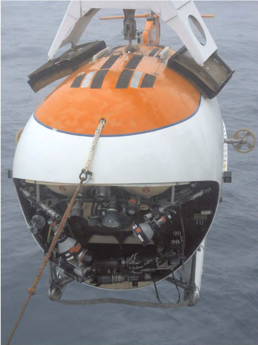
Figure 4.1. The Mir submersible is lowered into the water by a cable connected to the ship's winch. This view shows the versatile manipulator arms and the huge viewing port. The Mir project was developed by the USSR Academy of Sciences along with Design Bureau Lazurith. Built in 1987, Mir 1 and Mir 2 were designed and built by the Finnish company Rauma, Raepola's Oceanics subsidiary. In the mid 1990s and early 2000s, the submersibles were used by Canadian film director, James Cameron, to film the wreck of Titanic . On August 2nd, 2007, Russia used the submersibles to descend to the seabed under the Geographic North Pole (a depth of 4,261 m), a stunt that featured Mir 1 planting a (rustproof!) Russian flag on the ocean floor. Courtesy NOAA.
