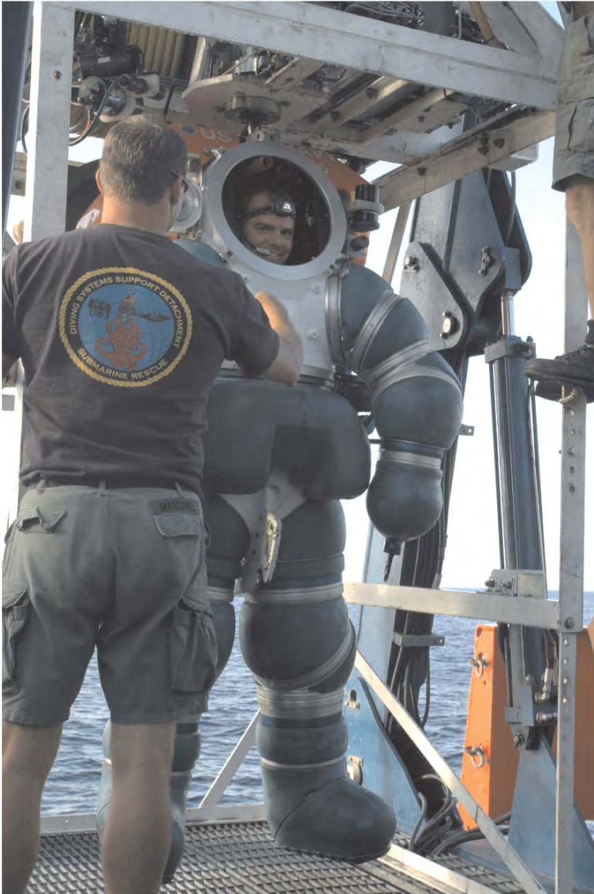
Figure 3.3. Chief Navy Diver Daniel P. Jackson is hoisted onboard the M/V Kellie Chouest following a successful certification dive of the Atmospheric Diving System (ADS 2000) off the coast of La Jolla, California, in August, 2006. Jackson's 600-m dive set a US Navy diving record. US Navy photo by Mass Communication Specialist Seaman Chelsea Kennedy. Courtesy United States Navy.
