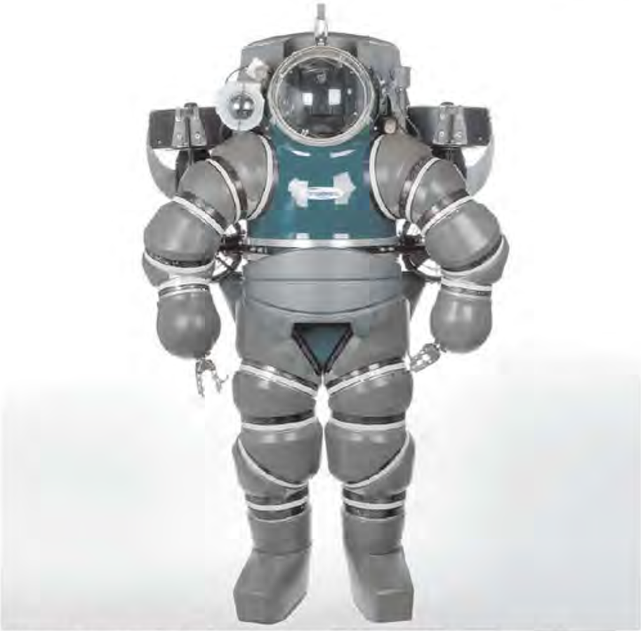
Figure 3.2. The OceanWorks atmospheric diving suit includes advanced life support monitoring and communications systems, which ensure diver safety. The life support system is a self-contained rebreather system that uses a carbon dioxide scrubber in conjunction with an onboard oxygen supply. The suit has 16 rotary joints and two foot-pedal-controlled thrusters to provide mobility. Its primary mission is submarine rescue. Courtesy OceanWorks.
