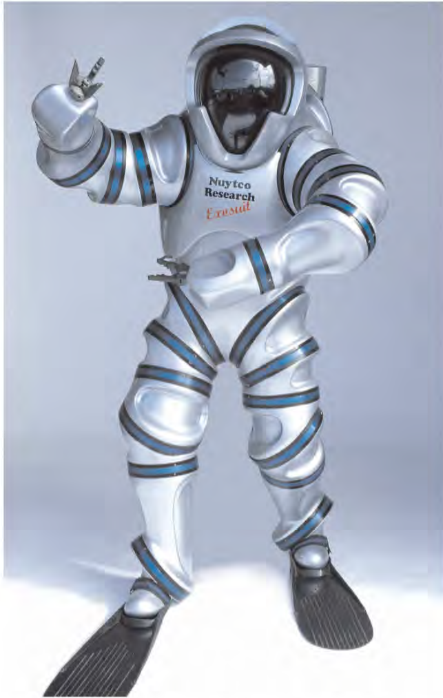
Figure 3.4. Exosuit is a swimmable atmospheric diving suit that enables divers to dive to 365 m while breathing air at atmospheric pressure for up to 3 days. A saturation diver diving to such depths would need to spend 8–10 days decompressing afterwards, whereas divers using the Exosuit require only 3–5 min recovery, independently of dive depth and duration. Covered in an A356-T6 aluminium alloy skin, the Exosuit is rated to 365 m, although its crush depth is over 600 m. Weighing 118 kg, the suit appears cumbersome, but appearances can be deceiving; the suit is extraordinarily mobile thanks to special joints and Prehensors that almost exactly mimic hand movements. Whereas a saturation chamber, bell, and gas storage might cost in excess of $4 million, the Exosuit costs just $250,000. One version of the suit is designed for submarine rescue. Surprisingly, despite being Canadian-built by Nuytco in North Vancouver, the Canadian Navy has no submarine rescue capability and has expressed no interest in acquiring the Exosuit. Courtesy Nuytco.
