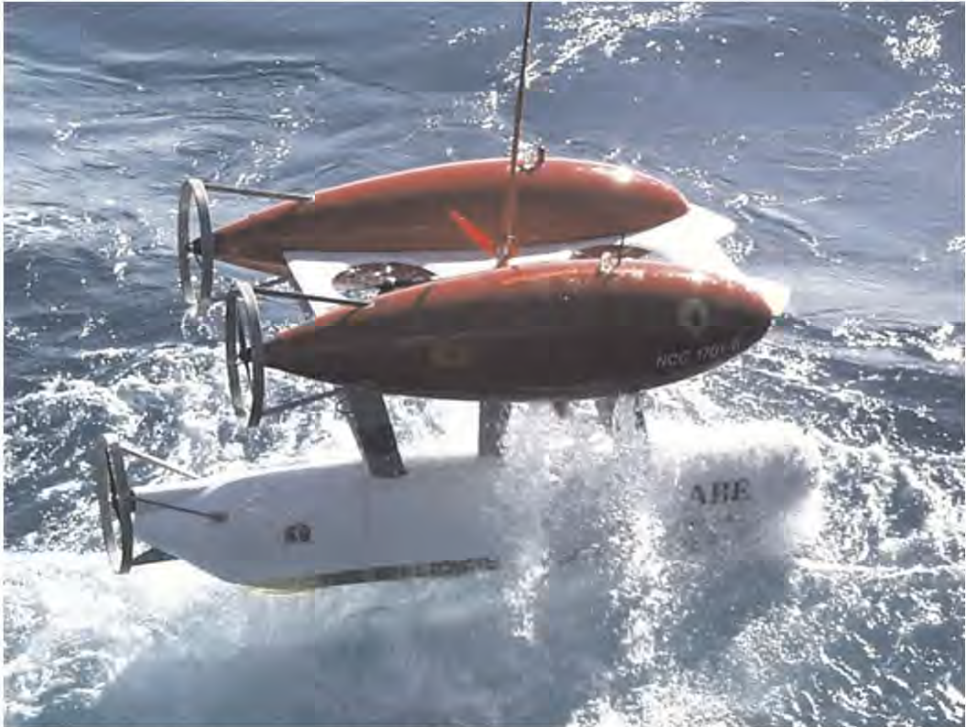
Figure 7.5. The Autonomous Benthic Explorer (ABE). Although hydrothermal plumes can be detected up to a distance of several kilometers from the emitting vent field with standard in-situ sensors, turbulent and chemically altered seawater makes location vent sites challenging, which is why AUVs such as the ABE are deployed. Courtesy Woods Hole Oceanographic Institution.
