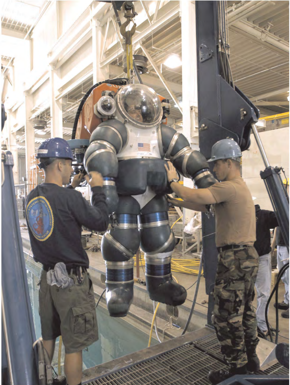
Figure 3.1. An atmospheric diving suit (ADS) is a one-man articulated submersible with articulated pressure joints. Some ADS systems can be used for dives of up to 700 m, and because the suit is maintained at 1 atmosphere, the dangers of decompression sickness are eliminated. ADS systems currently in use include the Newtsuit, the WASP, and the ADS2000. Courtesy United States Navy.
