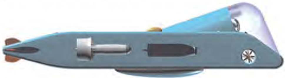
Figure 5.7. Deep Flight II. This revolutionary submersible has been designed but has yet to be built, and will be strong enough to dive down to 6,000 m. Courtesy Hawkes Ocean Technologies.
