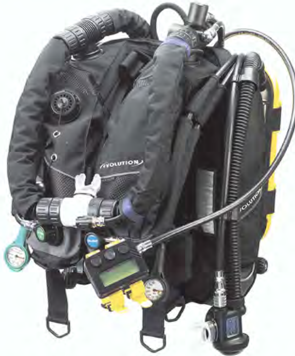
Figure 2.9. The Evolution showing the harness, wings, and hose. The system is an electronics-driven fully closed-circuit constant partial pressure of oxygen rebreather that provides the diver with a host of diving information via a heads-up display. It costs about US$10,000. Photo John Bantlin. Courtesy Ambient Pressure Diving.
