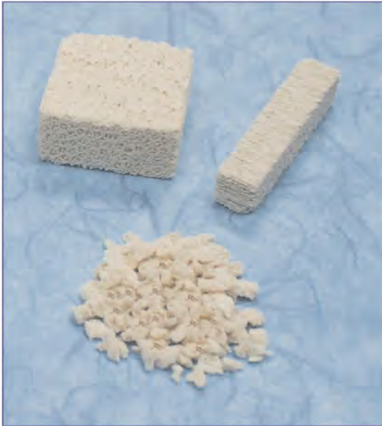
Figure 8.1. Hydroxyapatite can be produced from the exoskeletons of marine coral and is used as a bone graft to facilitate bone growth. Courtesy Wikimedia.
