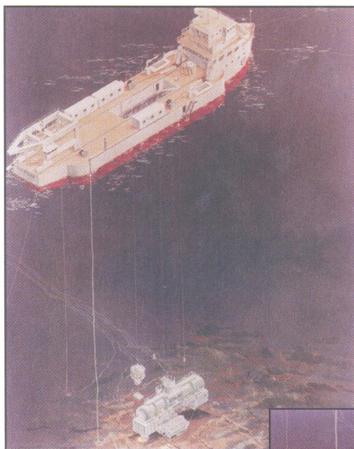
An artist's conception of Sealab III on the sea floor with the PTC (Personnel Transfer Capsule) stationed nearby. Note the diving station entrance ladder to the left and Observation Room on the far end to the right.
