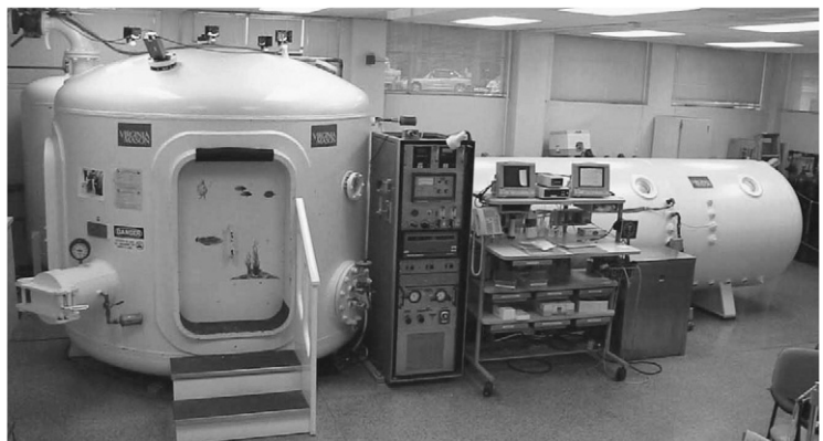
Figure 3.2 Dual-lock multiplace hyperbaric chamber, hybrid configuration with vertical and horizontal cylinders (in service 1970–2005, Virginia Mason Medical Center, Seattle).
