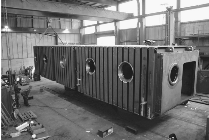
Figure 3.3 Rectangular multiplace hyperbaric chamber with external reinforcing ribs (installed 2006, Karolinska Institute, Stockholm, Sweden).
