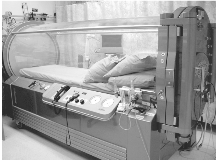
Figure 2.1 Monoplace hyperbaric chamber (Model 3200; Sechrist Industries, Inc., Anaheim, Calif). The internal diameter is 32.5 inches, the internal length is 90 inches, and weight is 1992 pounds. Gas flow through the chamber can be adjusted from 240 to 400 L/min. Maximum operating pressure is 3.0 ATA.
