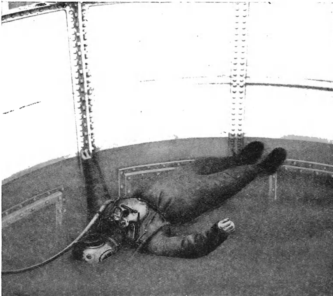
FIG. 26.—POSITION OF DIVER IN UNLACED DRESS AFTER BEING BLOWN UP.
