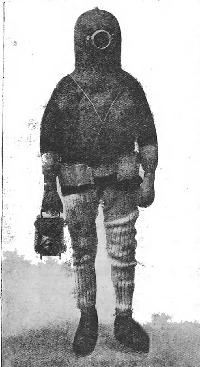
FIG. 66.—THE SUBMARINE DRESS WEIGHTED AND USED AS A DIVING DRESS FOR SHALLOW WATER (SIEBE, GORMAN AND CO.).
