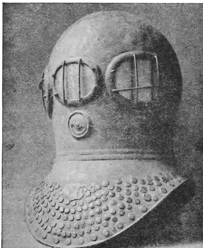
FIG. 12.—SIEBE'S FIRST DIVING HELMET.
