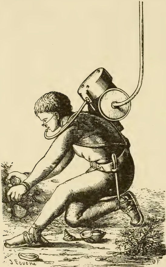
Fig. 8—Diver equipped with the Denayrouze regulator, helmet removed.
