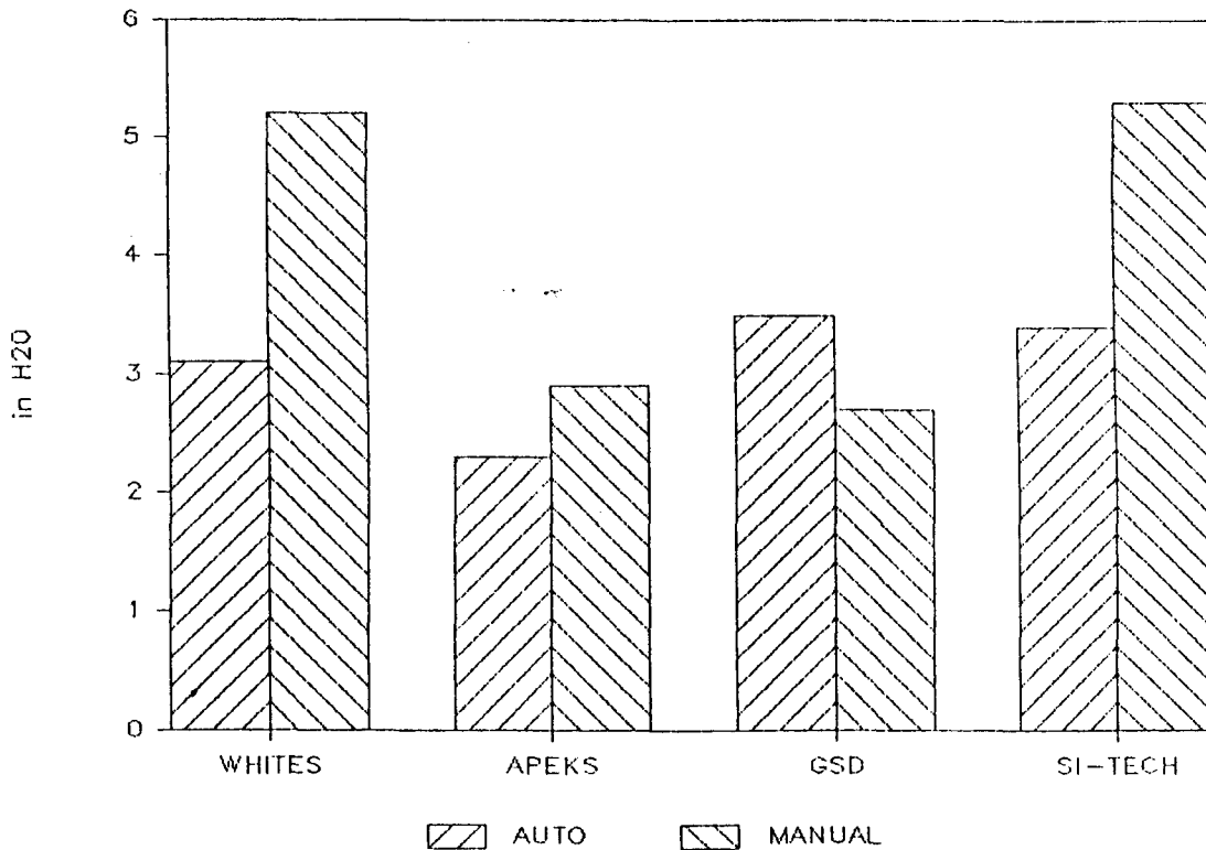
Figure 8. Pressure drop (inH 2 O), 5 cfm auto and manual operation
