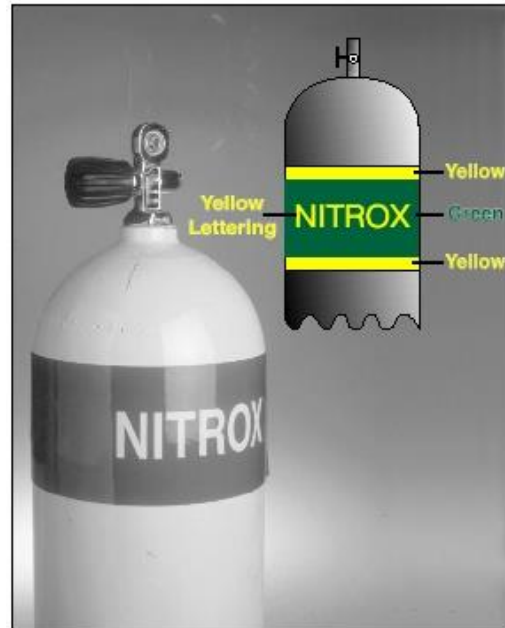
FIGURE 15.12 Single Tank with Nitrox Tank Wrap
