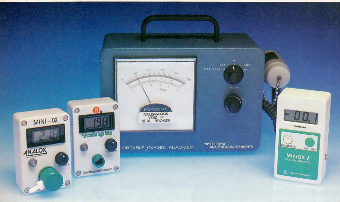
Figure 10-2. Oxygen analyzers. (From left) Analox Mini-O 2 , OMS Professional, Teledyne 320B, Miniox (Catalyst Research).
