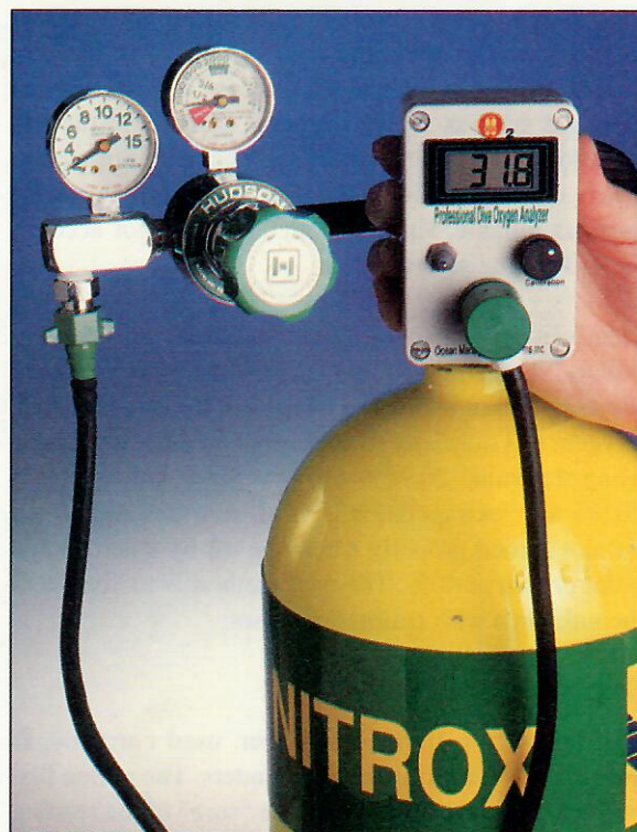
Figure 10-6. Gas sampling system using an oxygen analyzer with flow meter set to 2 lpm, analyzing an enriched air cylinder showing reading of 31.8%; this would be used as EAN 32 .
