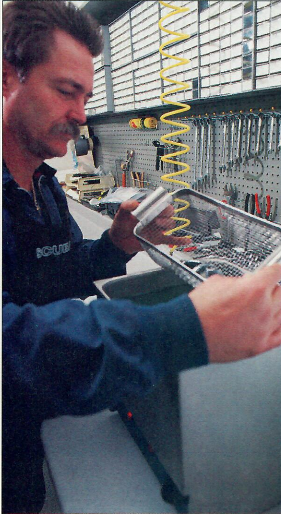
Figure 9-4. Service technician J.D. Selser prepares regulator parts for enriched air service.
