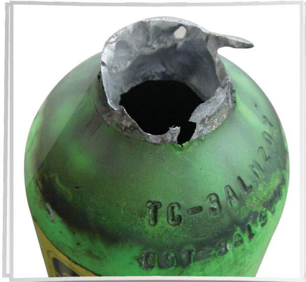
Figure 3-1: Contaminated Nitrox Cylinder after an explosion.
