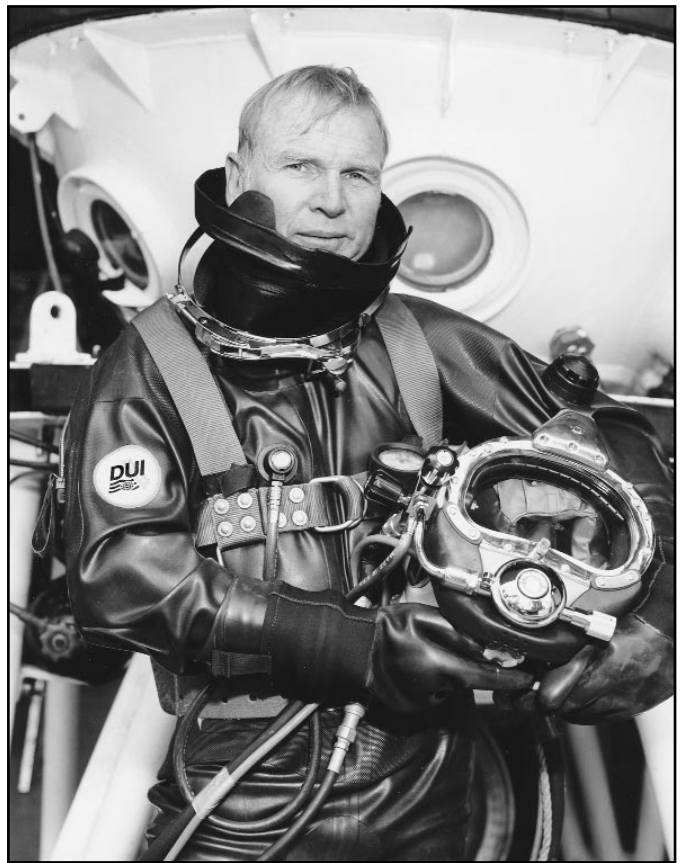
FIGURE 13.7 Full-Coverage Helmet with Dry Suit
