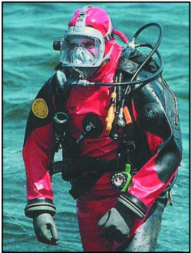
FIGURE 5.7 Heavy Duty Suit Made of Vulcanized Rubber
