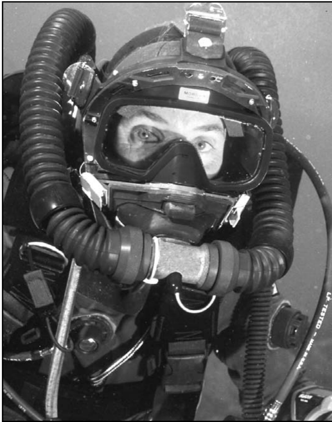
FIGURE 14.12 Full-Face Mask with a Closed-Circuit Rebreather
