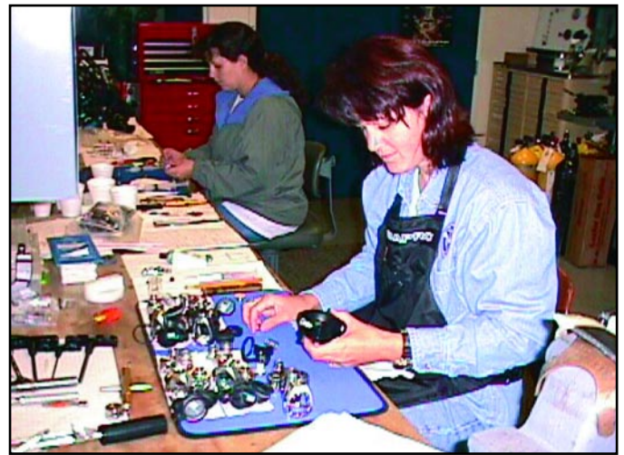
FIGURE 5.20 NOAA Technician Inspecting and Repairing Regulators
