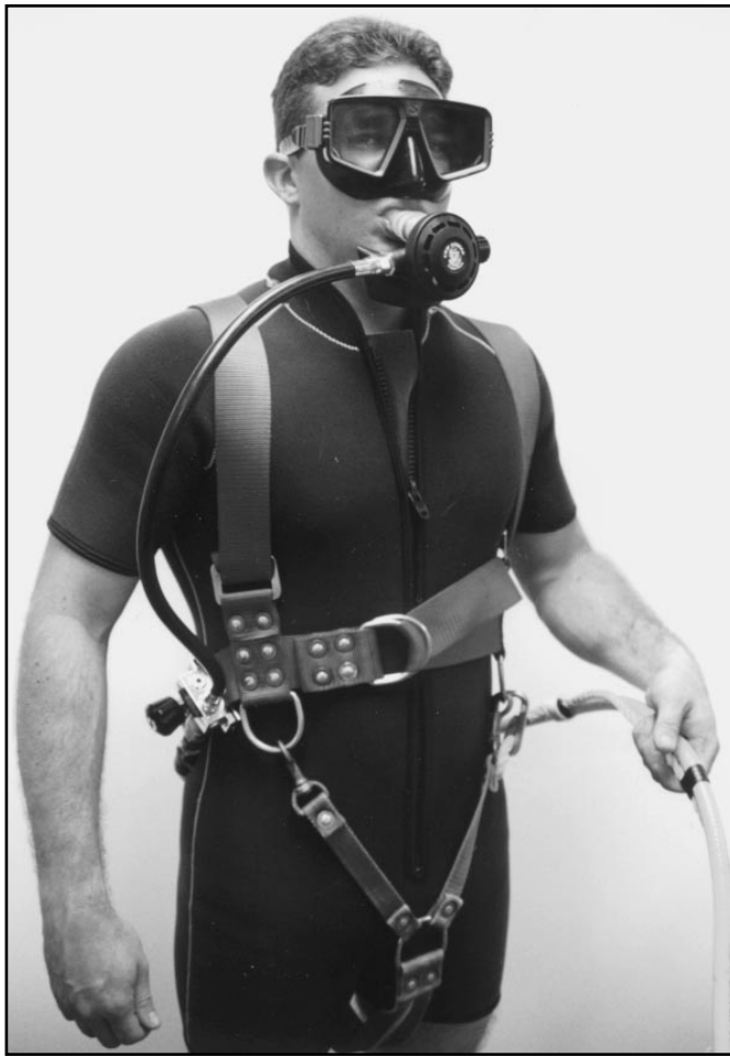
FIGURE 5.57 Hookah Diver With Second Stage and Lifeline Attached
