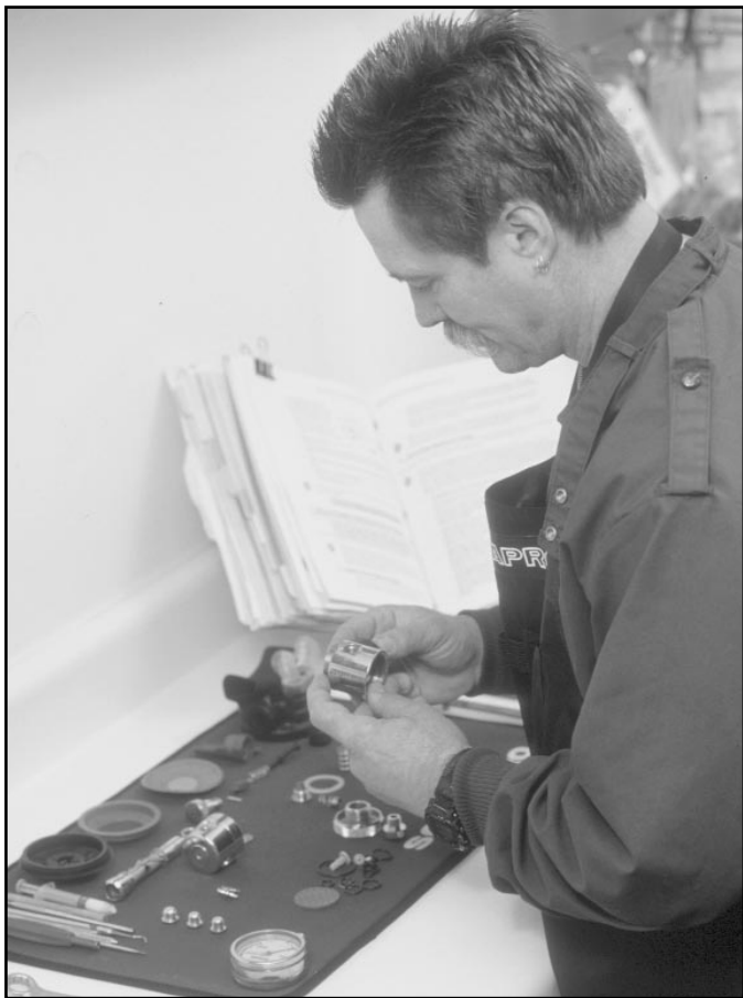
FIGURE 15.10 Preparation of Regulator Parts for Oxygen Service
