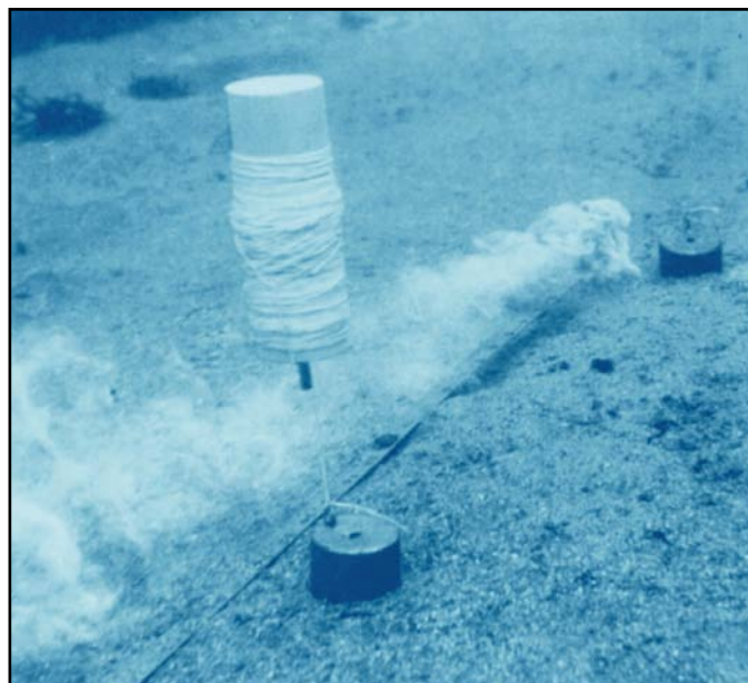
FIGURE 9.36 Dye-Tagged Water Moved by the Bottom Current
