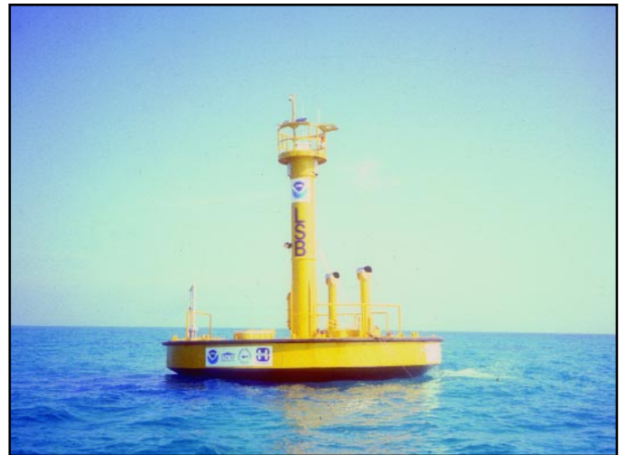
FIGURE 11.11 Life Support Buoy (LSB) for Aquarius 2000
