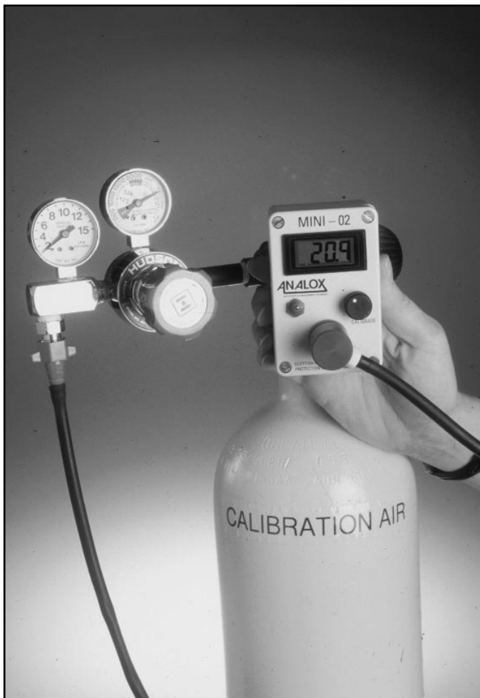
FIGURE 15.19 Oxygen Analyzer, with Flow Meter Set to 2 lpm
