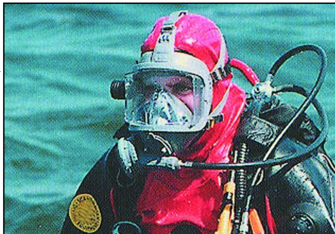
FIGURE 5.55 Full-Face Masks With Voice Communicators
