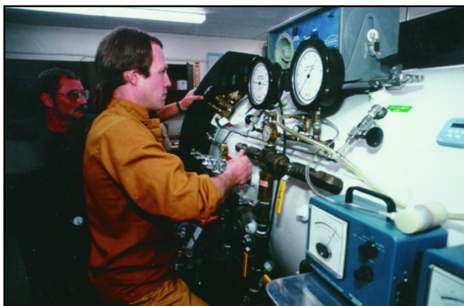
FIGURE 7.4 Diver Medical Technician (DMT) Pressurizing a Hyperbaric Chamber
