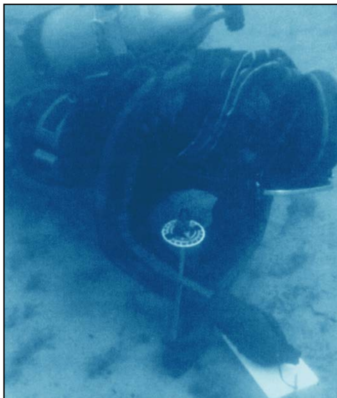
FIGURE 9.32 Taking a Vane Shear Measurement
