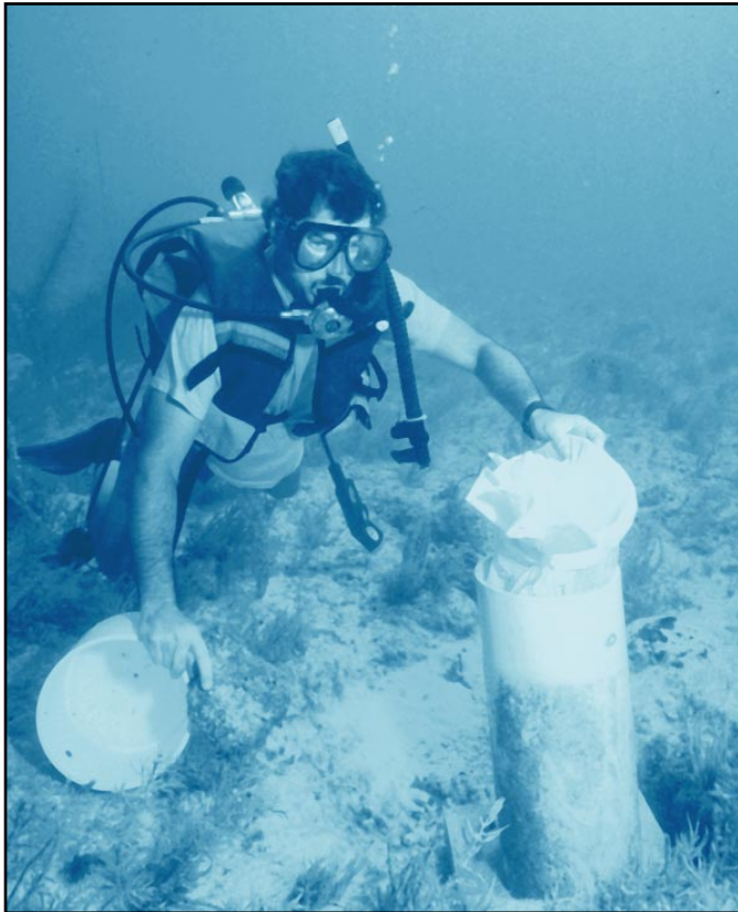
FIGURE 9.33 Deploying an Instrument Inside PVC Housing
