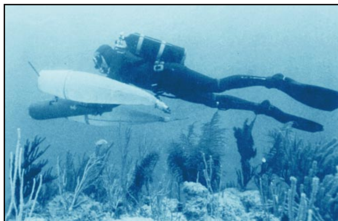
FIGURE 9.8 Hensen Egg Nets Mounted on Propulsion Vehicle
