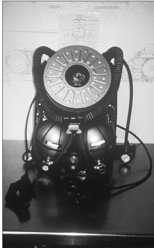
Figure 3-7. Closed-circuit rebreathing device showing counterlung and gas supply. (Photograph courtesy of Lee Somers.)
