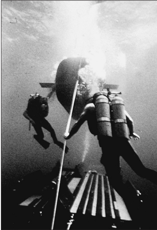
Figure 29-6. Launching the SDV from the Dry Deck Shelter. (Photograph courtesy of U.S. Navy.)
