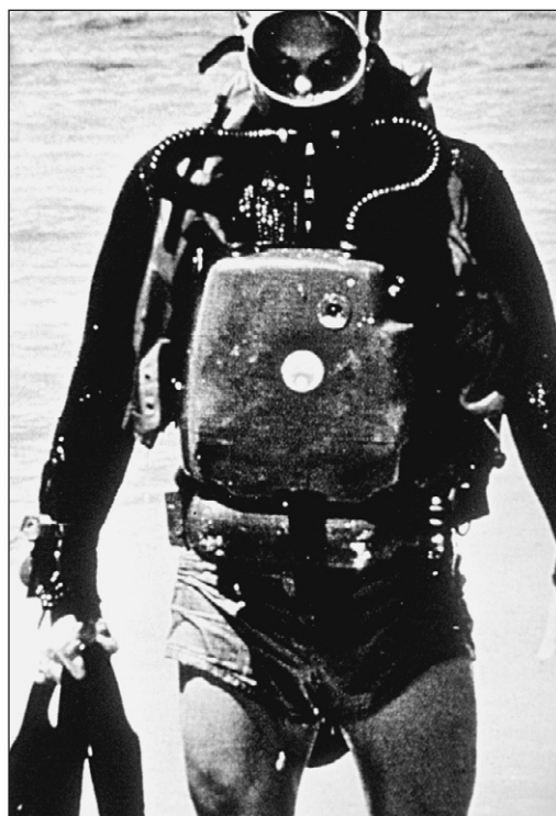
Figure 29-1. Diver wearing a Draeger LAR V UBA. (Photograph courtesy of U.S. Navy.)
