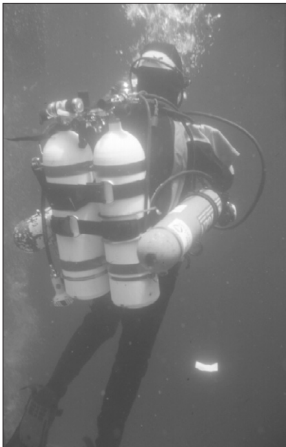
Figure 17-2. Deep air system with nitrox and oxygen. (Photograph courtesy of Mark Lonsdale.)
