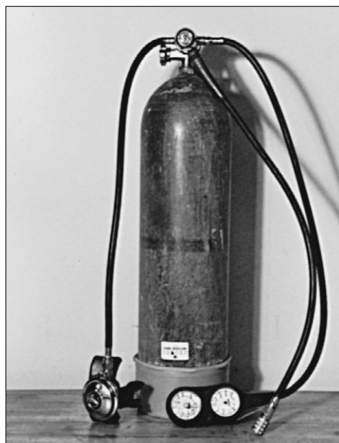
Figure 3-5. Typical open-circuit scuba apparatus consisting of a pressure cylinder, single-stage regulator, underwater tank pressure gauge, depth gauge, and spare hose for connecting to the buoyancy device.
