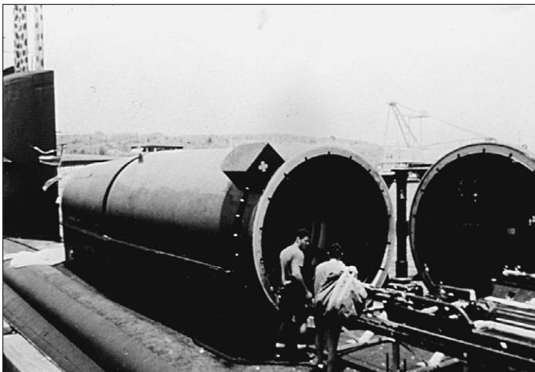
Figure 29-7. Dry Deck Shelter being loaded at pier-side. (Photograph courtesy of U.S. Navy.)
