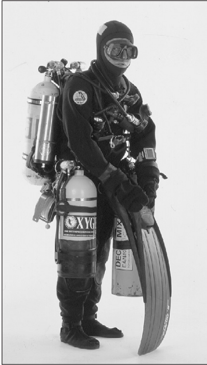
Figure 6–7. A technical diver shown wearing the complete outfit. Visible are dual back-mounted tanks, dual side-mounted tanks (each of these has a separate regulator, and there is a spare regulator on a long hose), a smaller tank of argon for suit inflation, a reel for managing independent ascent, lights, and a dive computer (mainly for logging), all on a hooded dry suit. Special thermal underwear and an adult diaper are also included with this outfit. (Courtesy of Dan Burton.)
