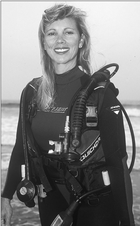
Figure 3–8. Low-profile buoyancy compensator with an integrated “quick draw” weight system and combined autoinflation air source. (Photograph courtesy of Mike Steidley.)
