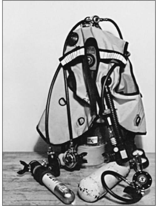
Figure 3-6. Clockwise from lower left: independent air supply, octopus, primary regulator, Air II, and pony bottle.
