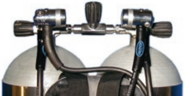
Close up view of hoses coming off the right and left posts.
