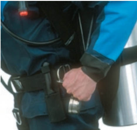
Left: SPG is clipped onto the left hip D-ring when not in use. Right: The SPG hose is long enough to allow viewing when unclipped.
