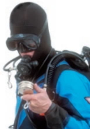
Left: SPG is clipped onto the left hip D-ring when not in use. Right: The SPG hose is long enough to allow viewing when unclipped.
