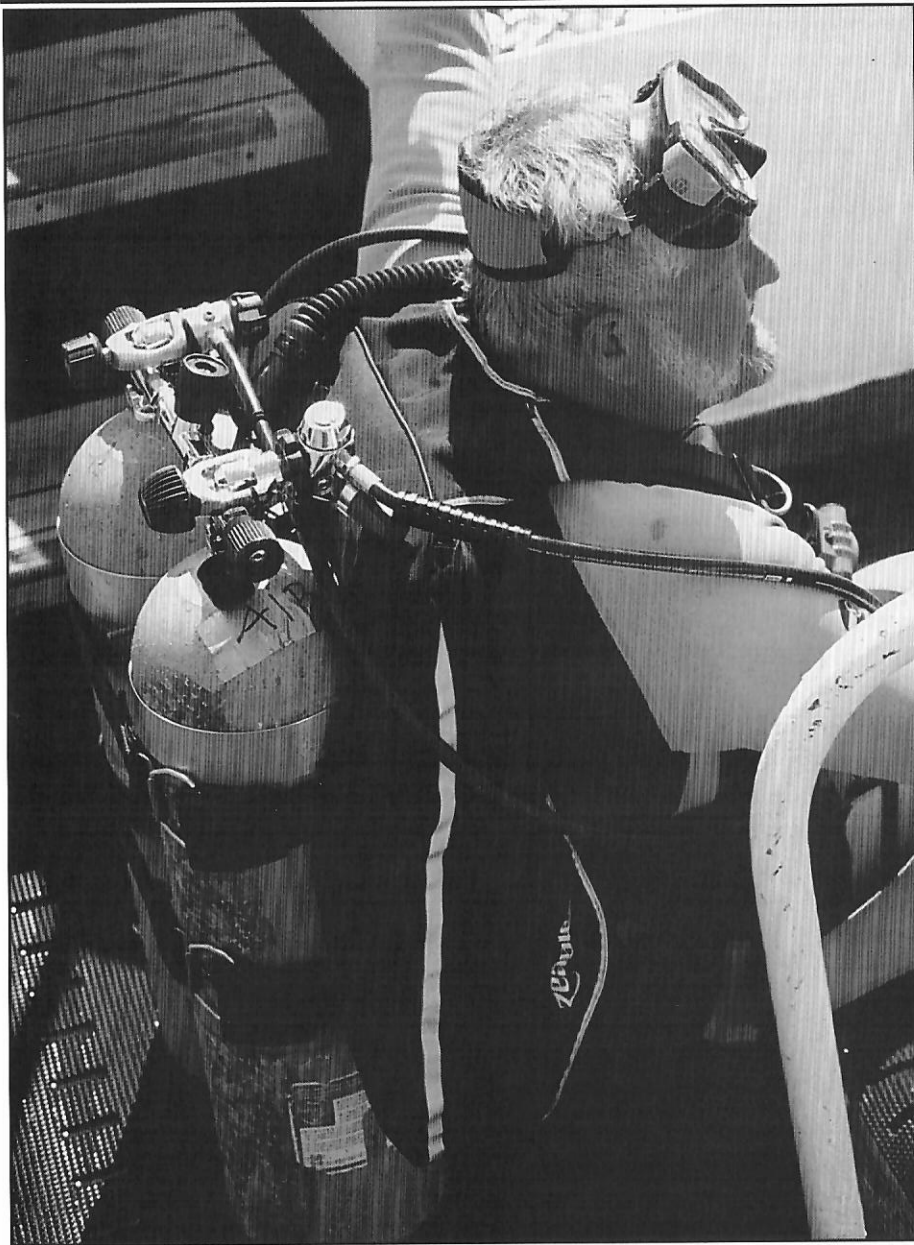
This diver is using two scuba cylinders joined together by an isolation manifold. The valve between the two cylinders allows either cylinder to be isolated from the other. Each cylinder has its own independent regulator. This arrangement provides the diver with many options in regards to how the air supply may be used and managed.
