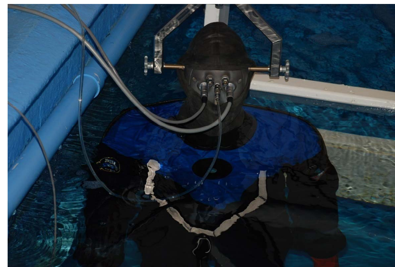
Figure 1. 21-zone thermal manikin outfitted in a tri-laminate drysuit
