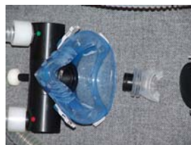
Fig 3: Close up of the SEA-LONG oral nasal mask and insert T-bit mouthpiece. The new hose clamps are also shown connecting the breathing hoses to the inspired (green dot) and expired (red dot) ports of the "T" valve.
