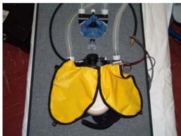
Fig. 1: Photo of the modified MBS 2000 closed circuit oxygen rebreather. During the dive trials oxygen was provided from D size (425 l) capacity cylinders attached to the high pressure supply whip with the over bottom pressure set at 125 psi.
