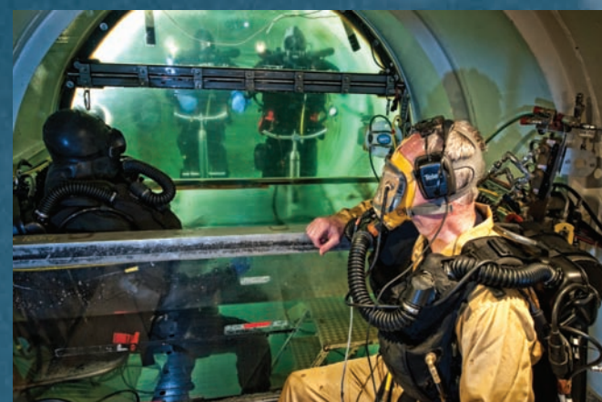
Figure 3. Four CUMA divers breathing trimix: 2 wet-working subjects on underwater bicycle ergometers (50 W; 5min cycling-5 min rest) wearing dry suits in 6-8°C water, one standby diver (resting, partially wet), and a team leader (dry, lightly working).
