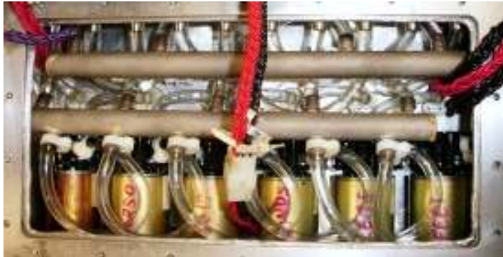
Gear Pump (B&D Pumps, Inc., UGP-2000P (24VDC)) Outlet and Inlet manifolds
