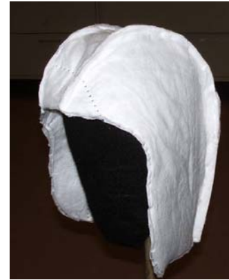
Aerogel hood with polymer film cover
