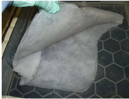
Gel infiltrated hood (solvent not yet extracted)
