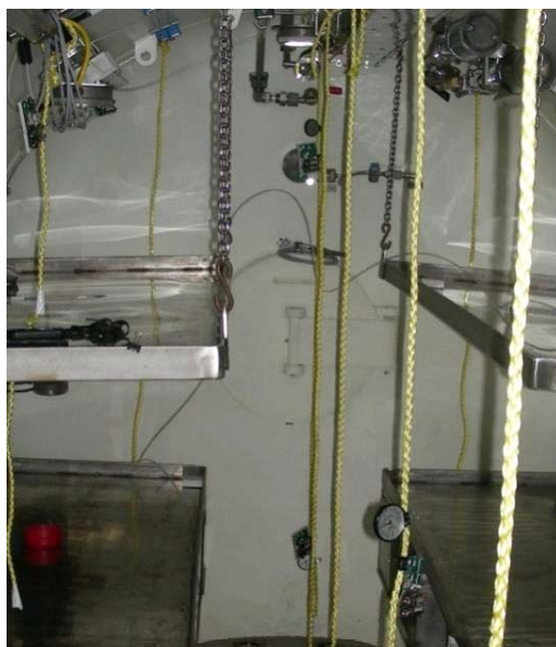
Left: Forward bulkhead in background with four bunks, several temperature sensors and gas temperature arrays (polypropylene rope) in foreground. Right: Infrared image of the same area shows thermal stratification on bulkhead and air
