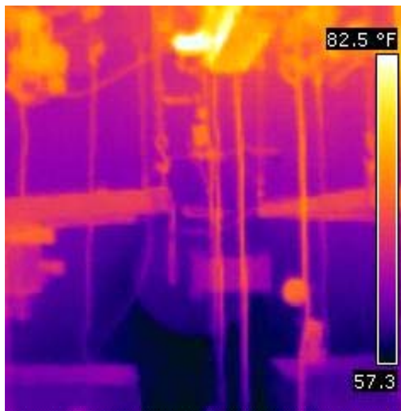
Left: Forward bulkhead in background with four bunks, several temperature sensors and gas temperature arrays (polypropylene rope) in foreground. Right: Infrared image of the same area shows thermal stratification on bulkhead and air
