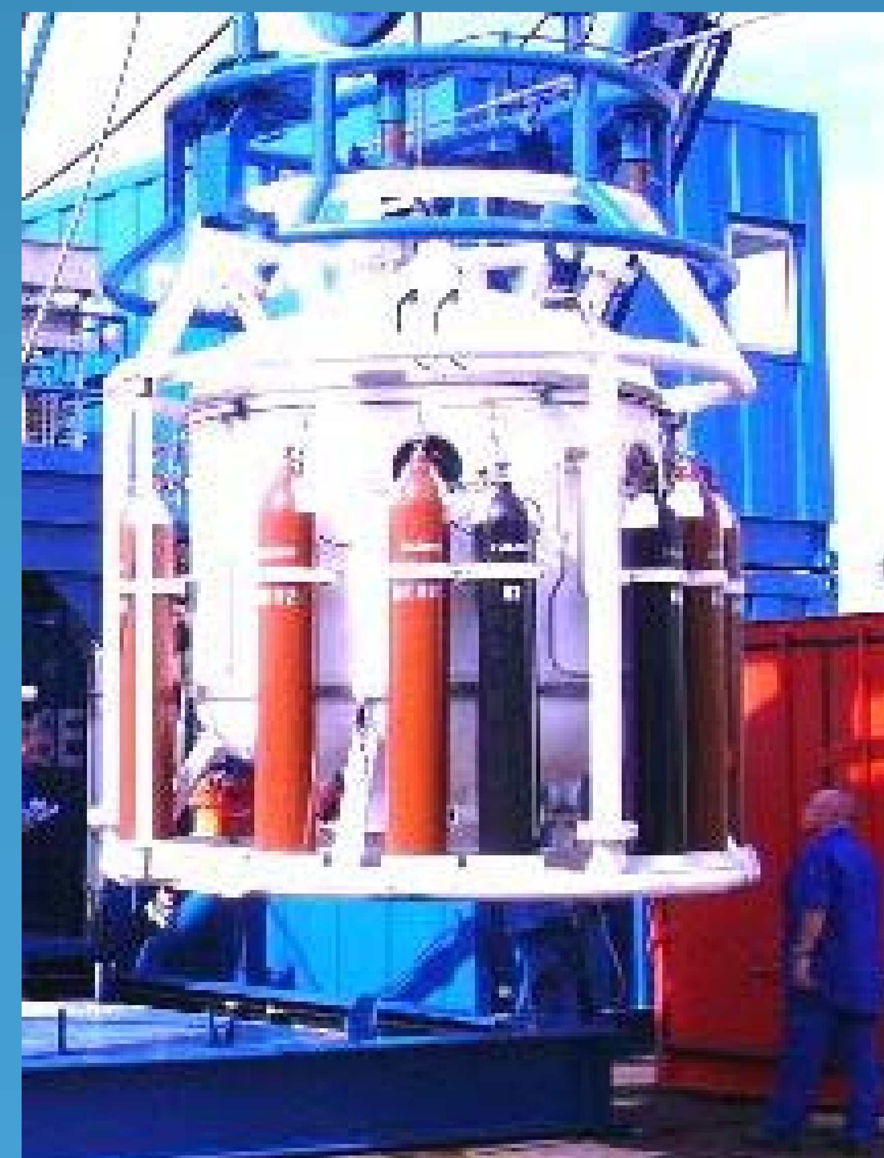
Transfer Bell: Used to transfer divers from work site to living quarters.
