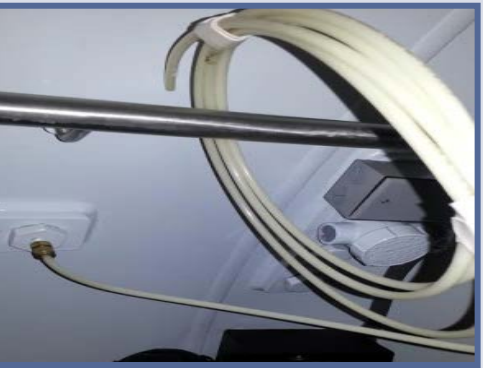
8) Differential valve connecting allowing ventilator to read outside ambient air pressure.
