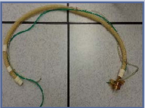
3) Tubing to connect the ventilator to the test lung.
