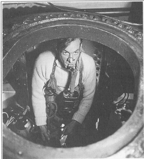
Welcome to the wet pot. Attendant above water breathing oxygen-nitrogen mixture to allow immediate decompression if necessary.
