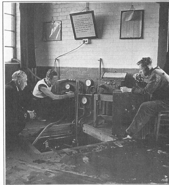
Wet Chamber sealed. Outside attendant gets "OK" signal. Pressurization starting.
