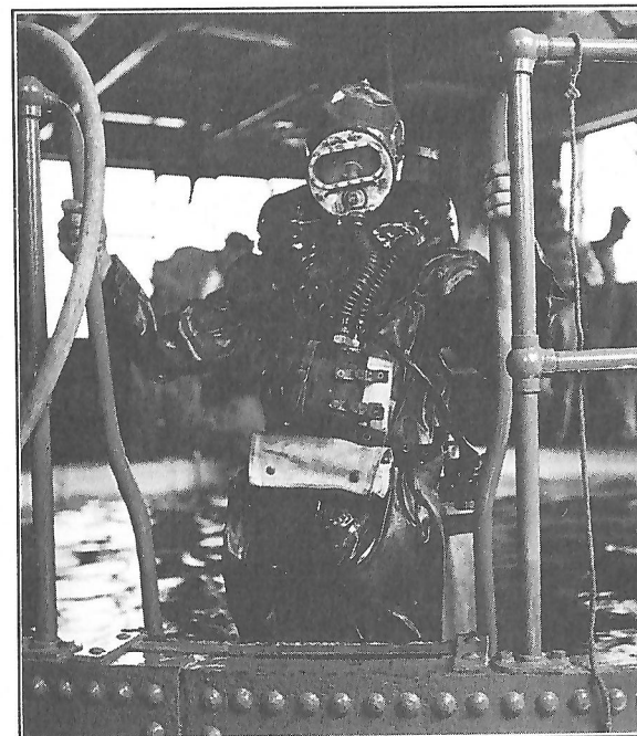
"Human Minesweeper" P-Parties. Oxygen-nitrogen mixture diver. Note raised counterlung in "ruff" position. Cylinder worn in "sword" position. Constant mass flow of mixture.
