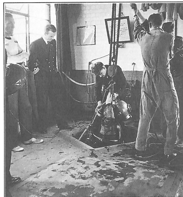
Rigid helmeted self-contained mixture diver being lowered into the "wet pot".
