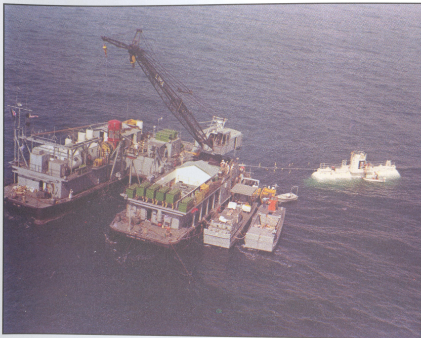
26 August 1965: 1,000 yards west of the Scripps Institute of Oceanography pier, Sealab II being prepared to descend 205 feet to the sea floor, with the Berkone in support.
