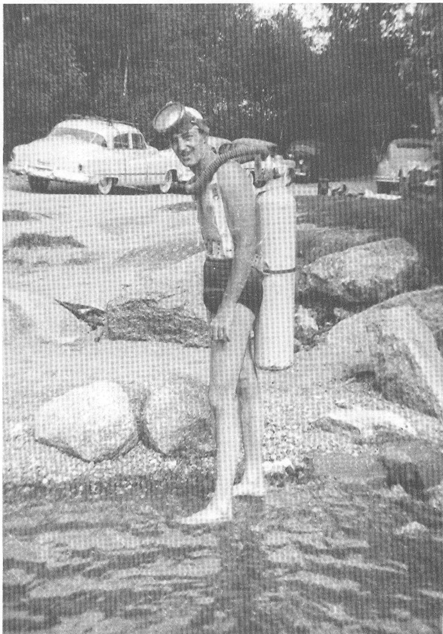
The author, wearing one of the famous "Big 99" salvage units. These 3,000 p.s.i. tanks are the world's largest self-contained single diving units. An Aqualung reserve valve and the Cousteau-Gagnan demand regulator complete the unit.
