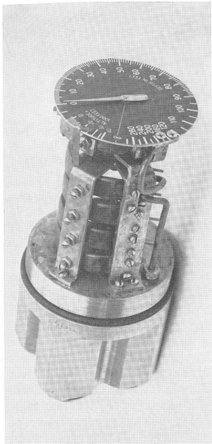
FIG. 16.6. Prototype Mk V S computer With pressure case removed to show dial pointers and Bourdon tube assembly.
