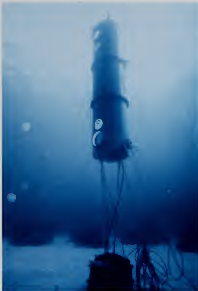
Figure 17-15D Undersea Instrument Chamber
