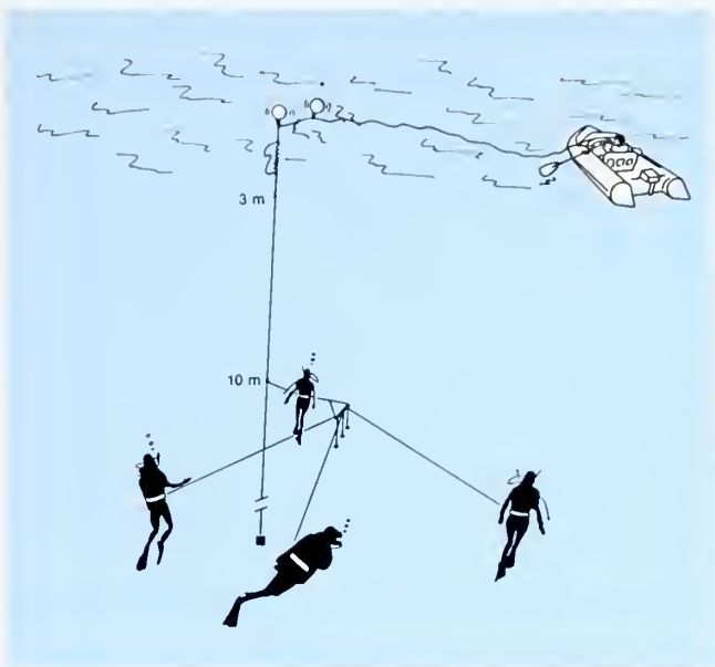
Figure 10-7 Down-line Array for Open-Ocean Diving
