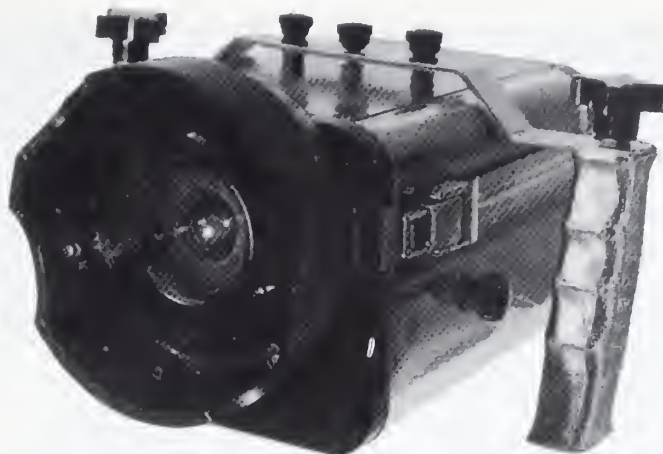
B. Underwater Housing With Angle Lens Attached
