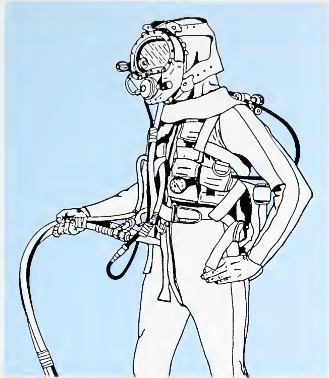
Figure 8-4 Surface-Supplied Diver In Lightweight Mask and Wet Suit
