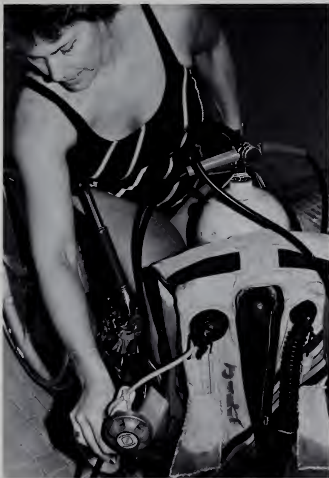
Figure A-9 Octopus Mounted for Ease of Use
