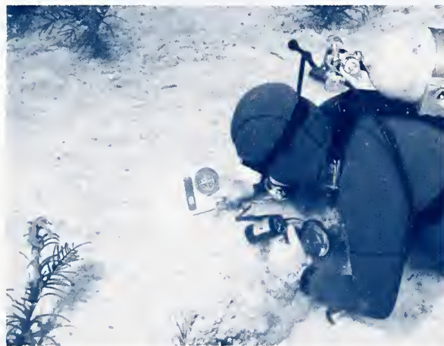
Figure 9-29 Geologist Measuring Dip (Inclination) of Rock Outcrop
