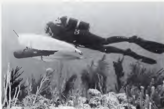
Figure 9-8 Hensen Egg Nets Mounted on a Single Diver Propulsion Vehicle
