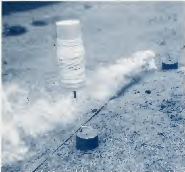
Figure 9-34 Dye-Tagged Water Being Moved by Bottom Current
