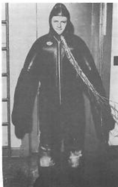
Maximal insulation. Diver wearing 4 x 3/4 in. foamed neoprene wet-suits was unable to maintain his body temperature in water at 4°C. (The wires are leads to skin thermocouples). Photo: U.S. Nav. Med. Res. Inst.
