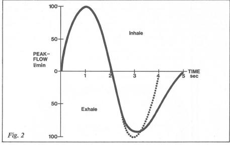
The dotted line shows a perfect sine curve, which is what a machine would do. The important part is that for work underwater when you are consuming 30 l/min, you need a regulator which delivers at least 100 l/min if you are not to beat the regulator.
