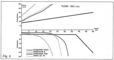
The reason for the dotted line for the 50/10 was the fact that this went on to free flow because of the extremely high peak-flow and it was not until 10 m that a reading could be taken.
