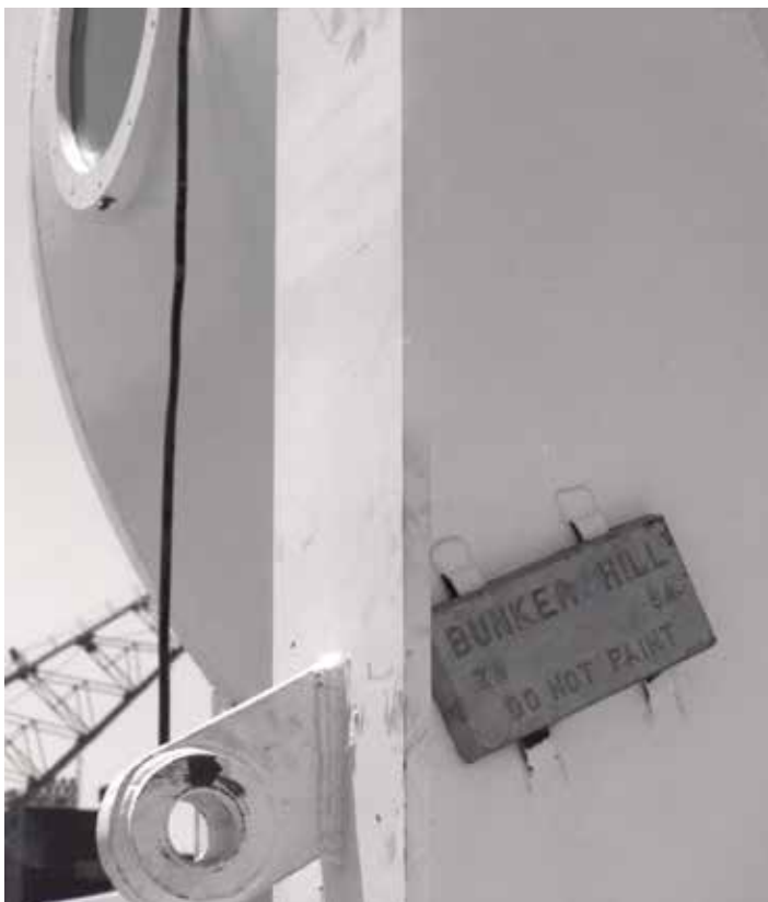
Fig. 2: Anode grade zinc plates are added for corrosion control. (Official photograph, U.S. Navy)
