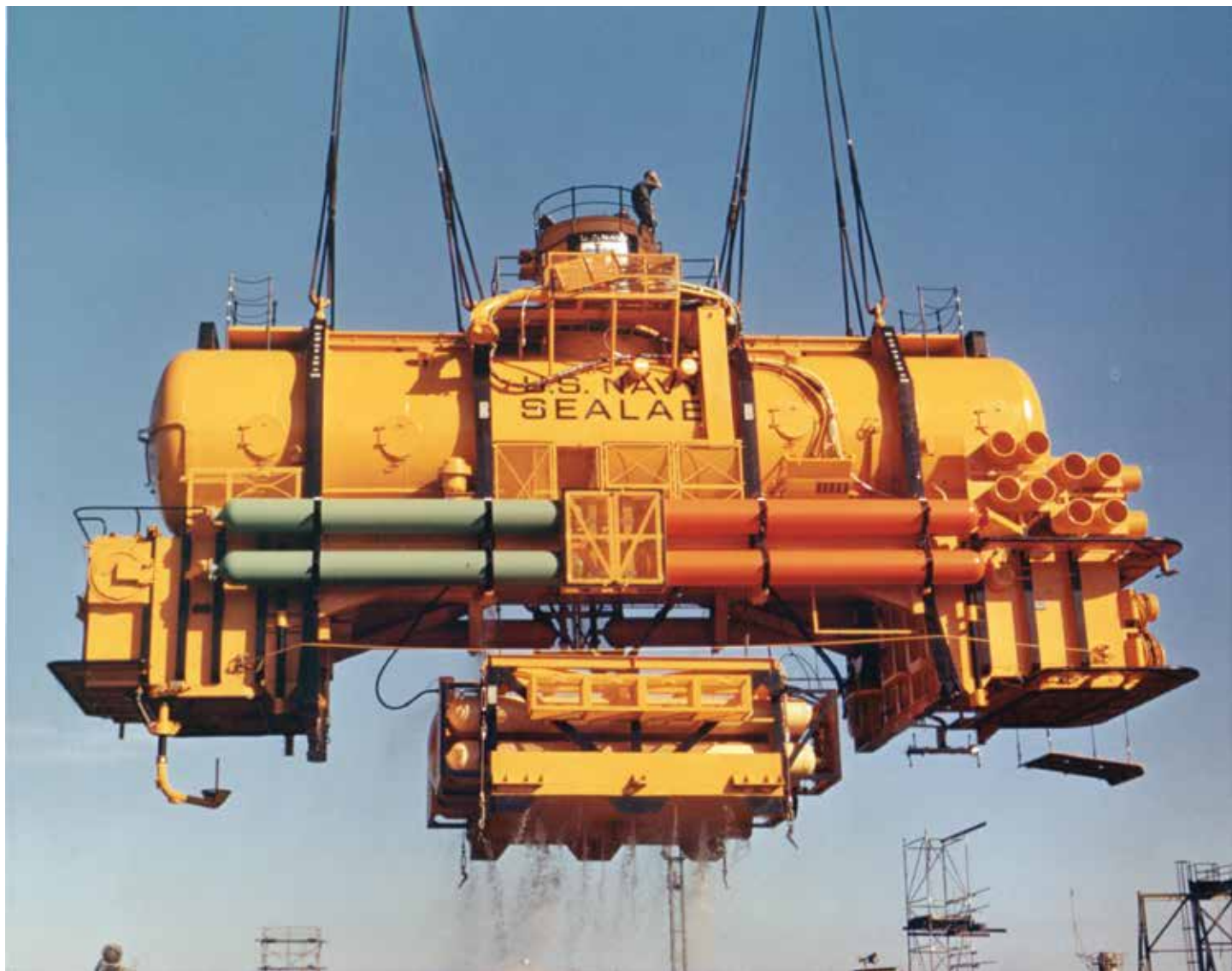
Figure 5: SEALAB III incorporated extensive modifications to the SEALAB II habitat. (Official photograph, U.S. Navy)
