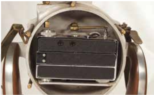
An interior shot showing the Argus C3 camera in place.
