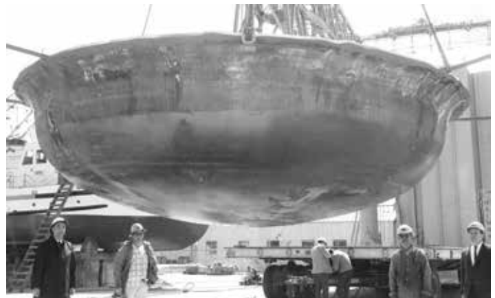
SEALAB II end bell immediately after being removed from shaping die. (Official U.S. Navy photograph.)
