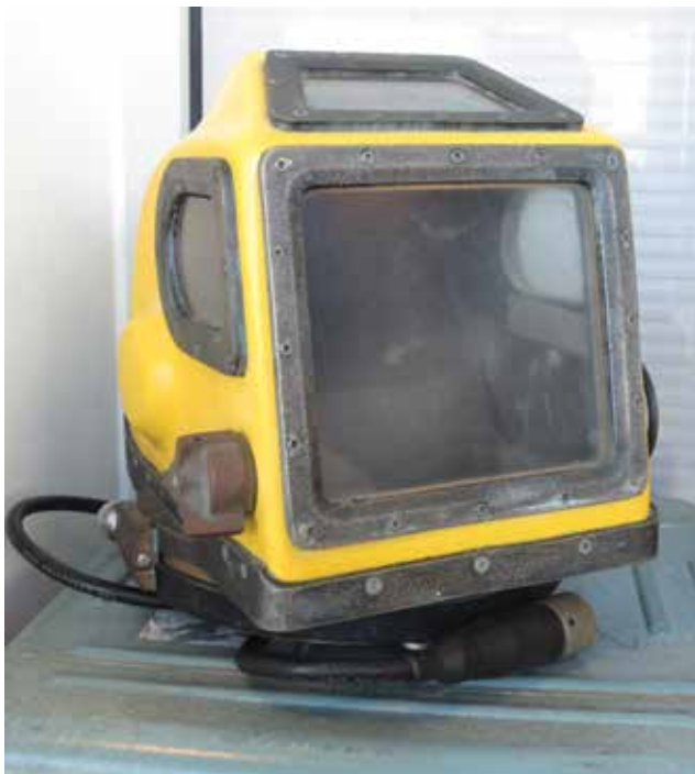
USN Mark XII helmet by Morse Diving Equipment Co. Inc. of Boston, Mass. This fiberglass helmet replaced the famed USN Mark V helmet as the primary USN helmet in the early 1980's.
