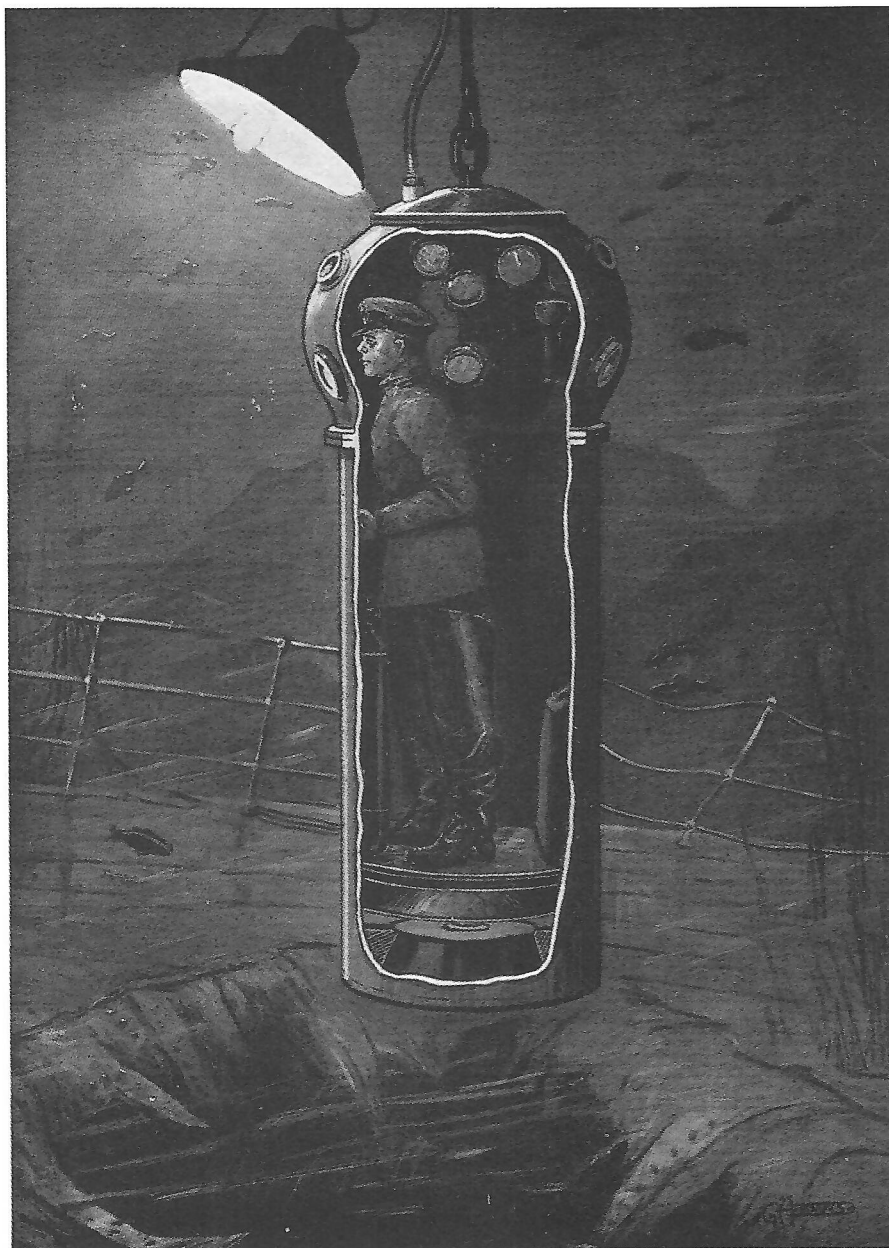
Fig. 177. Siebe, Gorman submarine observation chamber without buoyancy tank, and provided with air regenerating apparatus
