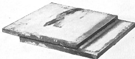
Fig. 190. Steel plates welded under water
