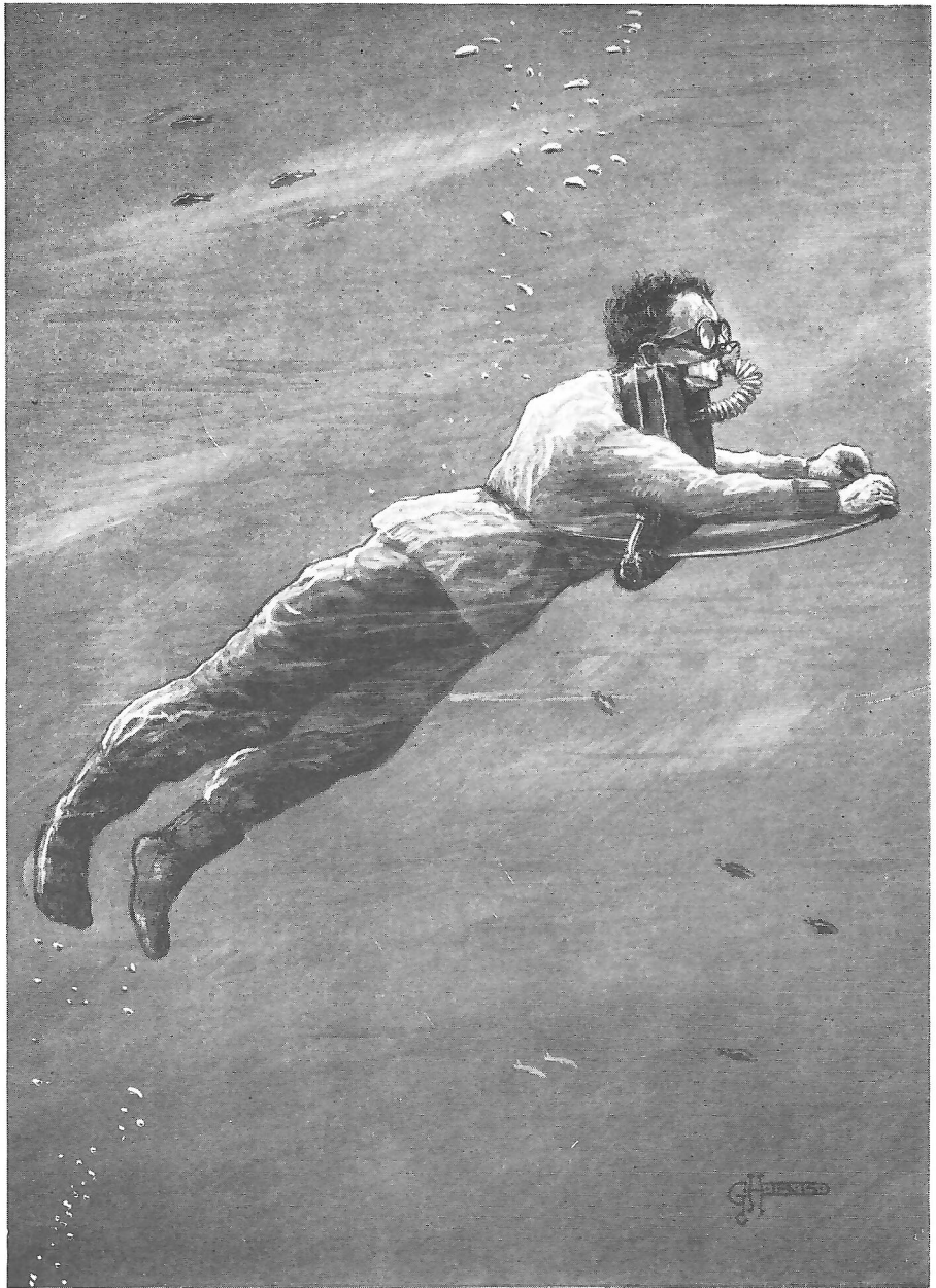
Fig. 252. Man with Davis apparatus ascending—with check-vane extended in order to retard speed
