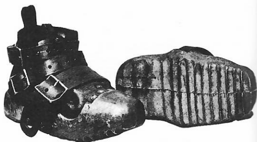
Fig. 87. Diver's boots with all-metal goloshes and renewable leather uppers
