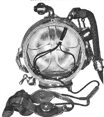
Fig. 83. Receivers on separate head-band. Transmitter in helmet. British Admiralty pattern
