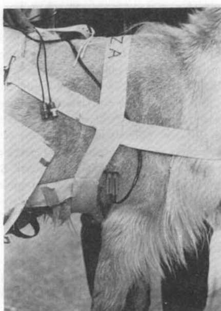
Figs. A, B, C, and D. Doppler ultrasonic transducer (5 MHz) and cuff showing A , how transducer fits into nylon cuff with stainless steel clip, and B , lead arrangement. Small connectors are miniature co-axial connectors (Amphenol Sub-Miniax 27-109) mounted on a circuit board which is then potted with epoxy and silicon rubber into the dacron felt pack; C , dacron pack which was stitched subdermally; dermal tissue healed into the dacron felt surface, providing an antiseptic seal and allowing convenient access to the animal as shown D , on animal with harness and strain-relieved leads.
