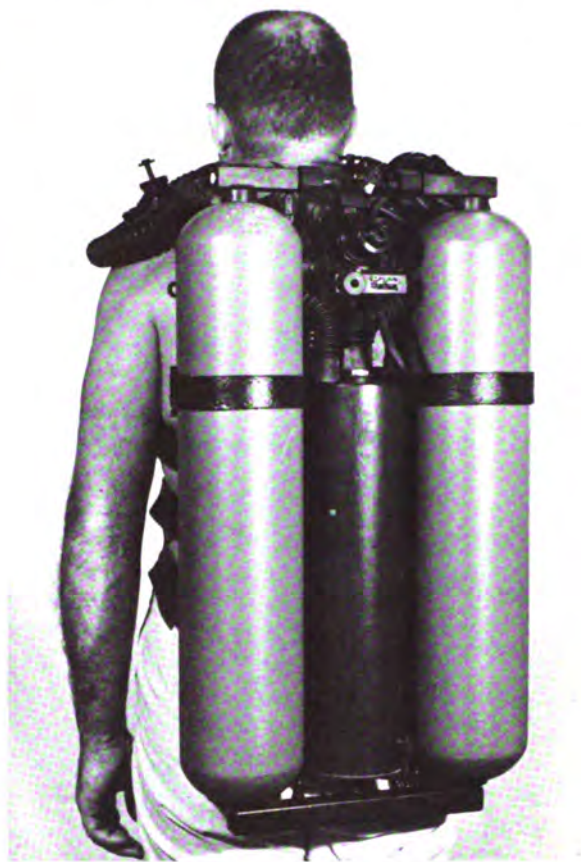
FIGURE 3-35.—Pure-oxygen recirculating, underwater breathing apparatus (back view).
