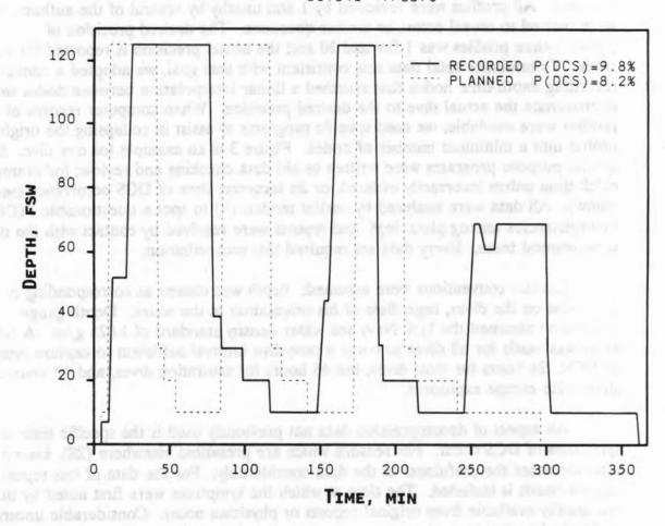
Figure 2. Comparison of an experimental dive profile between the data of the automatic depth recorder and the tabulated entry in the report for the planned profile. Repeated delays in descent because of divers' ear problems produced over an hour delay.
