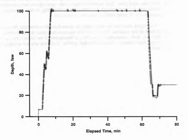
Figure 3. Comparison of raw depth-time record (points) with the simplified node structure in the final data record (line segments).
