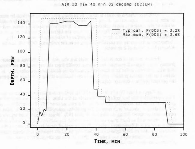
Figure 1. Comparison of a typical diving profile (solid line) with a literal interpretation of the dive based on the depth and time entry chosen for a decompression schedule.
