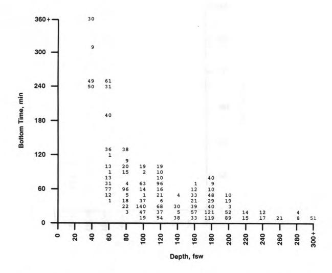
Figure 7. Distribution of air-equivalent depths and bottom times for all single non-saturation dives.
